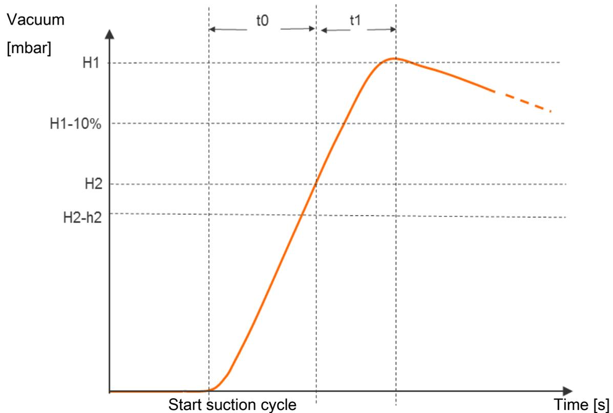
The specified value for the max. permitted evacuation time can be set in the configuration menu with the parameter [E - l] or via IO-Link [0x006B]. Setting the value to [000] (= off) deactivates monitoring. The maximum permitted evacuation time setting is 9.99 s.
