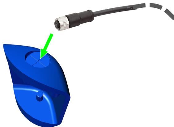
3. Connect the cable either by its loose strands to the appropriate positions on the terminal block (4.1) or by the M12 connector (4.2).
