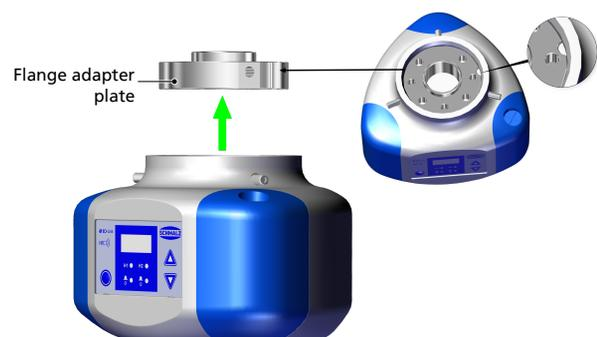
2. Attach the CobotPump using three radial set screws (M5x16) tightened to 0.6 Nm.
