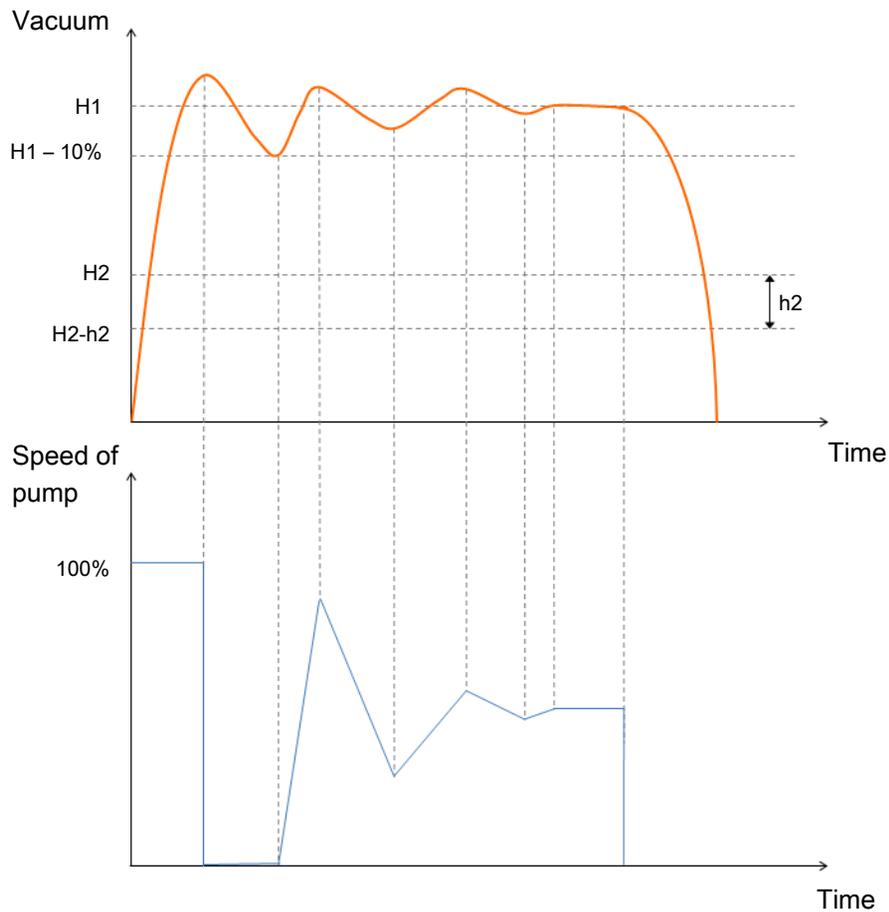
The output OUT2 (parts control) is set to "on" when the limit value H2 is reached. If the limit value H2-h2 is underrun, then the output is set to "off."
