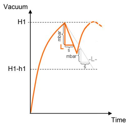
The permitted leakage value  $-L-$  can be set in the configuration menu with the parameter  $[-L-]$  or via IO-Link.
