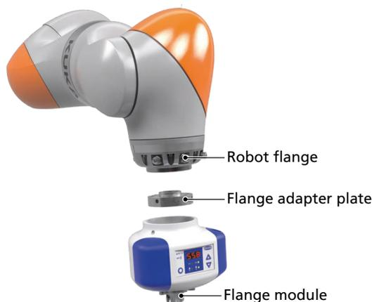
The CobotPump can be attached to a collaborative robot using a replaceable flange adapter plate. The markings on the flange and on the housing of the CobotPump must be observed, as these determine the orientation of the display and the suction cup on the robot.
