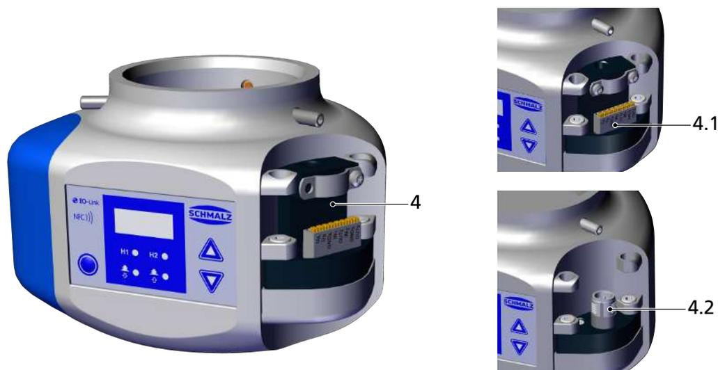
The CobotPump is electrically connected to the power supply and for input and output signaling purposes via the interface at item 4. The connection can be established using a flexible cable connection for device versions with a terminal block (4.1) or an 8-pole M12 connector (4.2).
