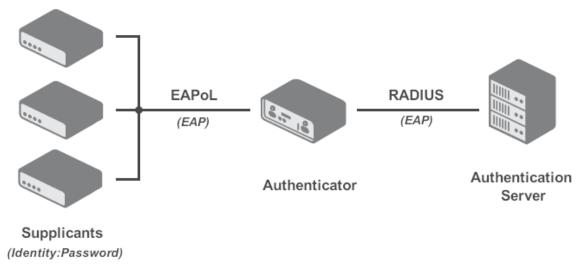
Figure 15: IEEE 802.1X Functional Diagram
