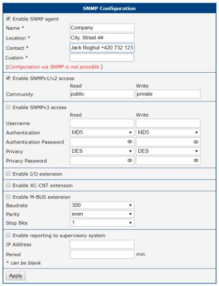
Figure 77: SNMP Configuration Example
