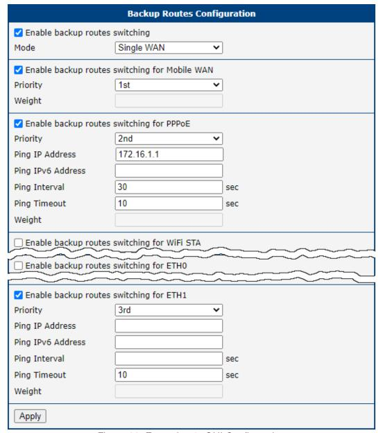
Figure 38: Example #3: GUI Configuration
