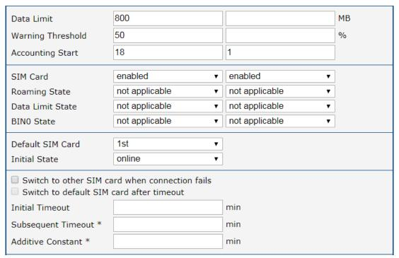
Figure 29: Configuration for SIM card switching Example 2
