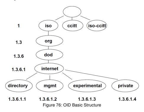
The SNMP values that are specific for Advantech routers create the tree starting at OID = .1.3.6.1.4.1.30140. You interpret the OID in the following manner:
