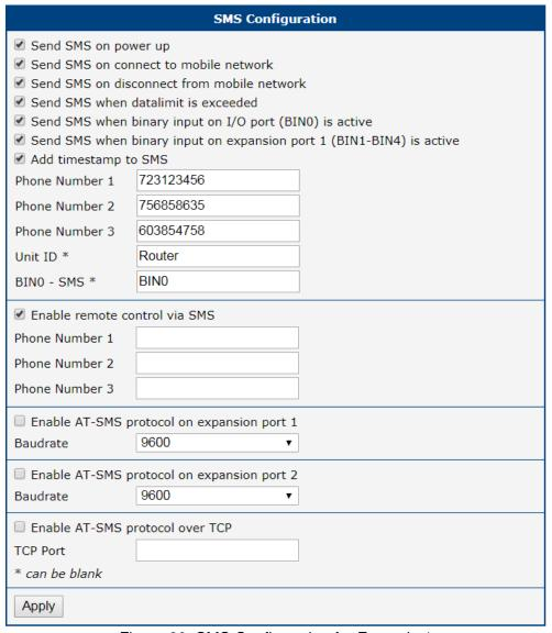
Figure 80: SMS Configuration for Example 1
