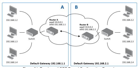
Figure 64: Topology of GRE Tunnel Configuration Example
