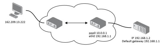
Figure 51: Topology for NAT Configuration Example 1
