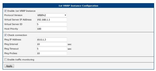
Figure 25: Example of VRRP Configuration – Backup Router
