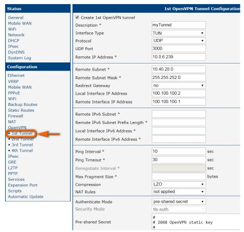
Figure 128: Secure networks interconnection – OpenVPN configuration
