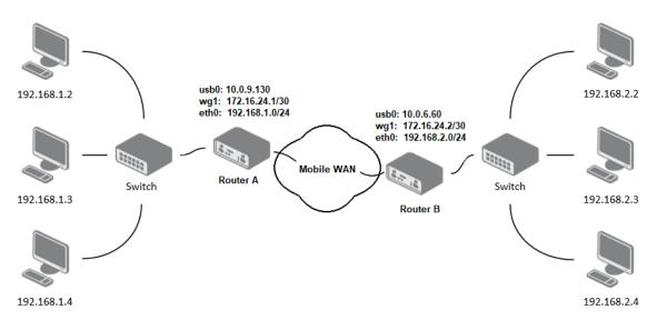
Figure 60: Topology of WireGuard Configuration Example
