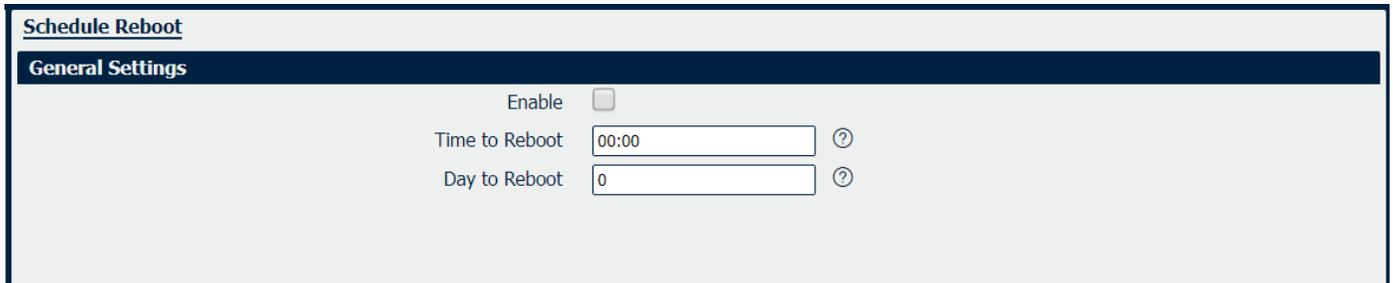
The screenshot shows a web interface for configuring the 'Schedule Reboot' feature. At the top, there is a header 'Schedule Reboot' and a sub-header 'General Settings'. Below this, there are three configuration options: 'Enable' with an unchecked checkbox, 'Time to Reboot' with a text input field containing '00:00', and 'Day to Reboot' with a text input field containing '0'. Each input field has a help icon (a question mark in a circle) to its right.
