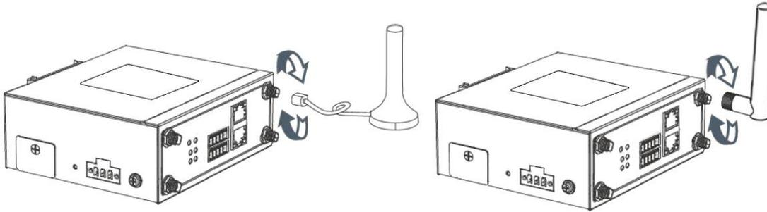
**NOTE:** NR500 router supports dual antennas with MAIN and AUX connectors. MAIN connector is for data receiving and transmission. AUX connector is for enhancing signal strength, which cannot be used separately.
