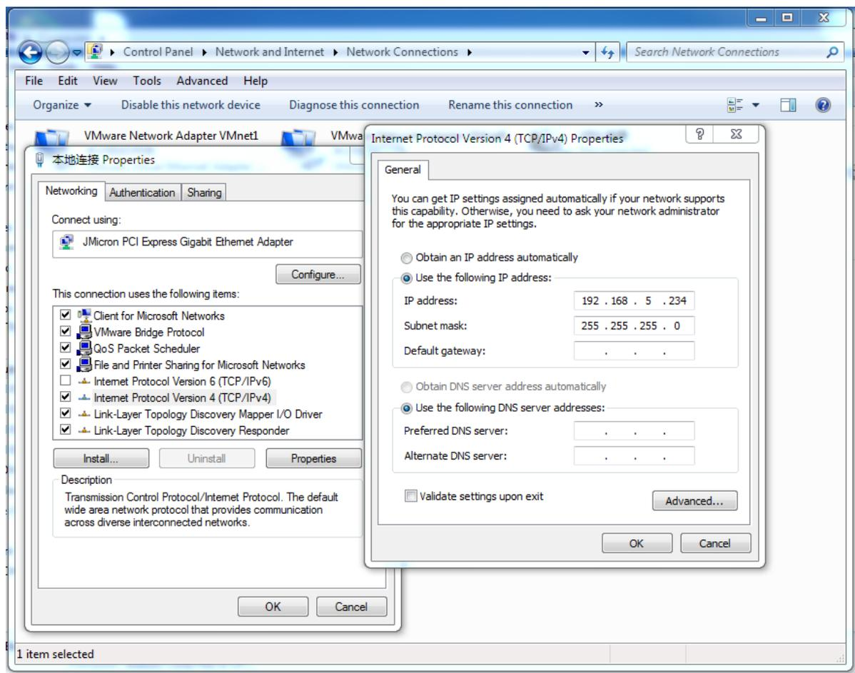
click "**Use the following IP address**" to assign a static IP manually within the same subnet of the router.
