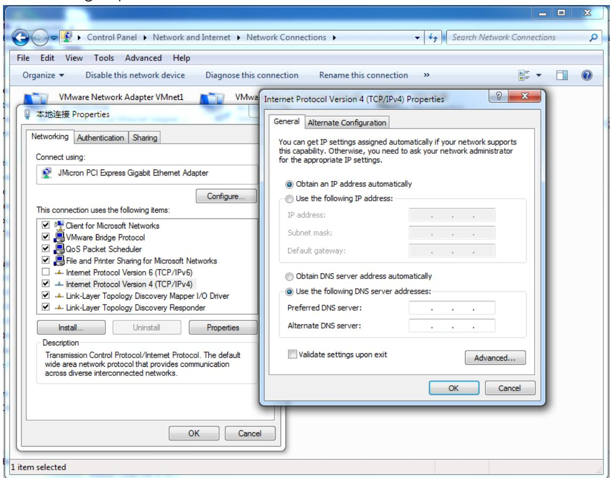
select **Start » Control Panel » Network Connections**. Right click **Local Area Connection** and select **Properties** to open the configuration dialog box for Local Area Connection. Select **Internet Protocol (TCP/IP)** and click **Properties** to open the TCP/IP configuration window. On the General tab, select **Obtain an IP address automatically** and **Obtain DNS server address automatically**. Click **OK** to complete TCP/IP configuration.
