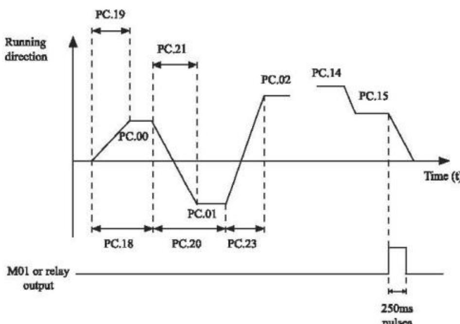
Figure 4-28 Simple PLC when used as frequency source
