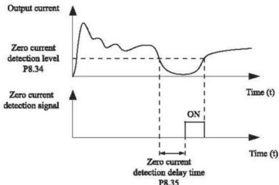
Figure 4-19 Zero current detection
