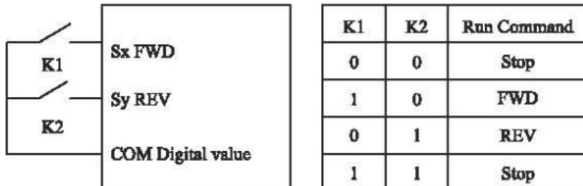
Figure 4-8 Setting of two-line mode1
