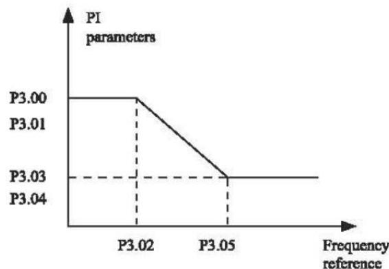
**Figure 4-4 Relationship between running frequency and PI parameters**
