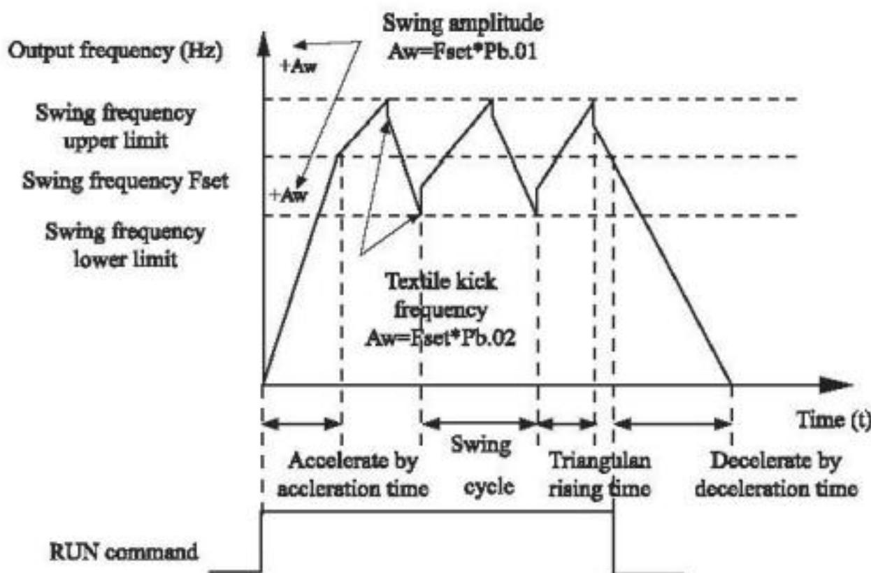
Figure 4-26 Swing frequency control
