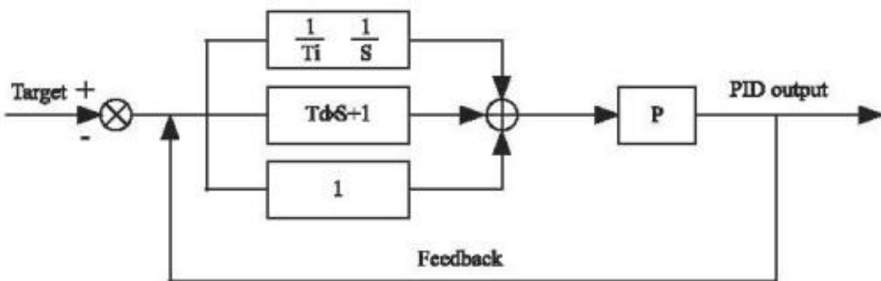
**Figure 4-23 Principle block diagram of PID control**
