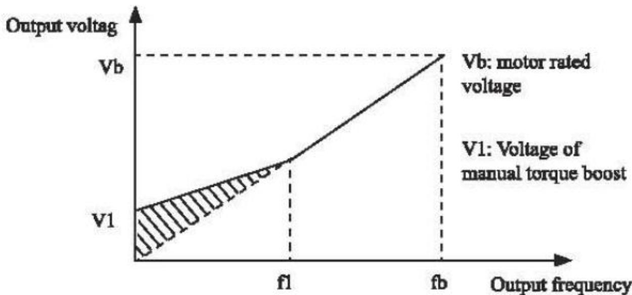
Figure 4-5 Manual torque boost
