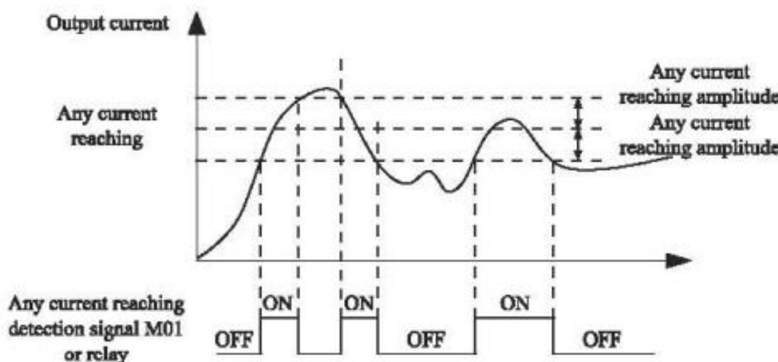
Figure 4-21 Any current reaching detection
