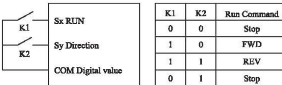
Figure 4-9 Setting of two-line mode 1
