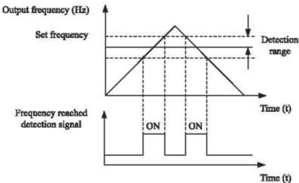
Figure 4-15 Detection range of frequency reached
