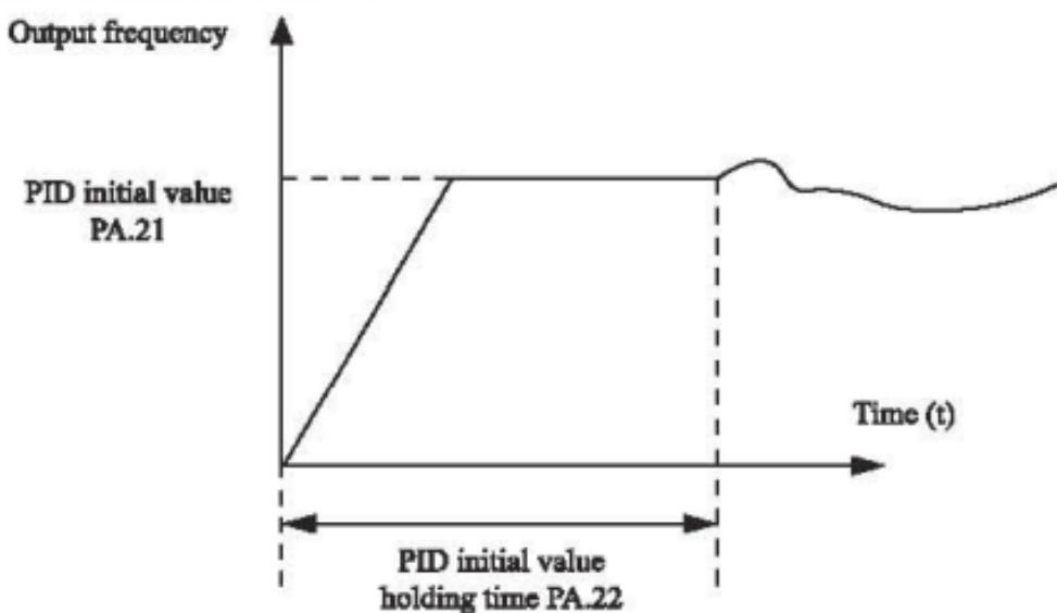
Figure 4-25 PID initial value function
