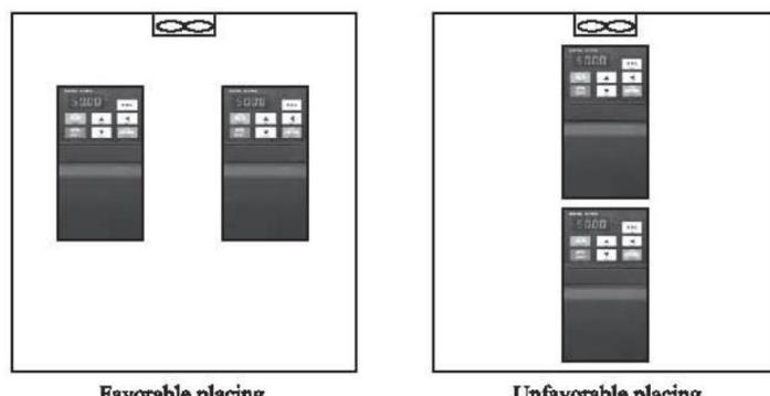
② If multiple inverters are installed in one control cabinet, please leave enough clearances and take cooling measure.
