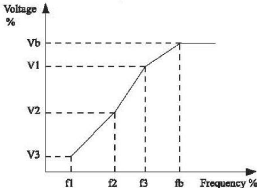
Figure 4-6 Setting of multi-point V/F curve
