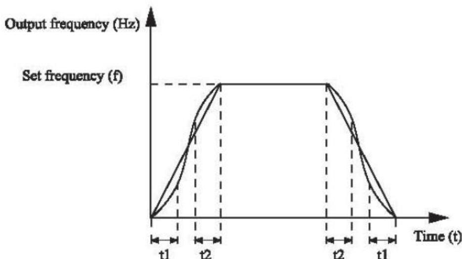
Figure 4-2 S-curve acceleration/deceleration A
