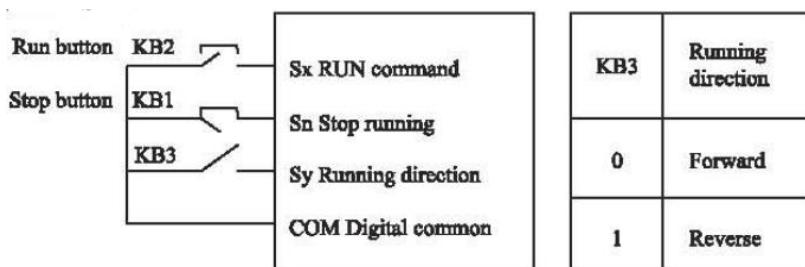
Figure 4-10-2 Setting of three-line mode 2
