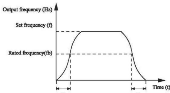
Figure 4-1 S-curve acceleration/deceleration B
