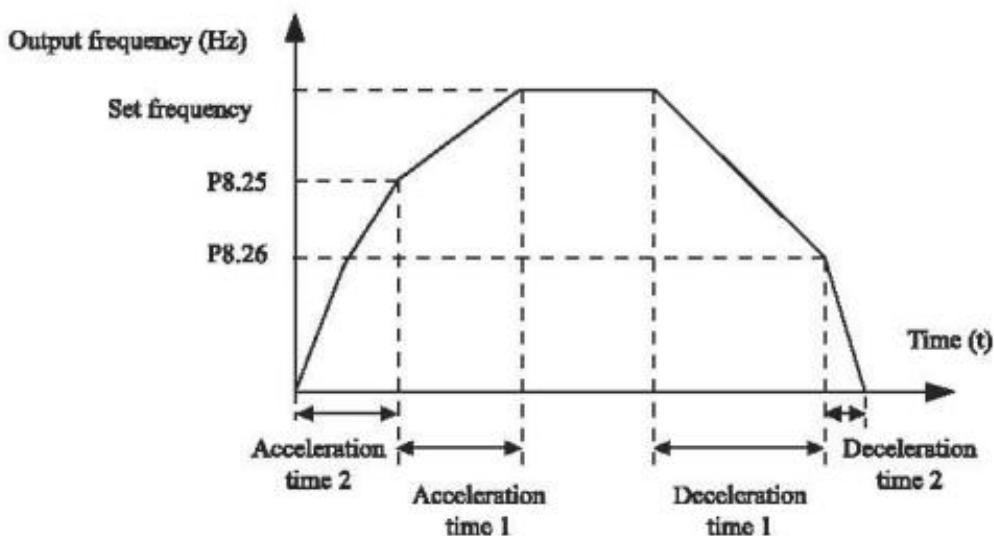
Figure 4-17 Acceleration/deceleration time switchover
