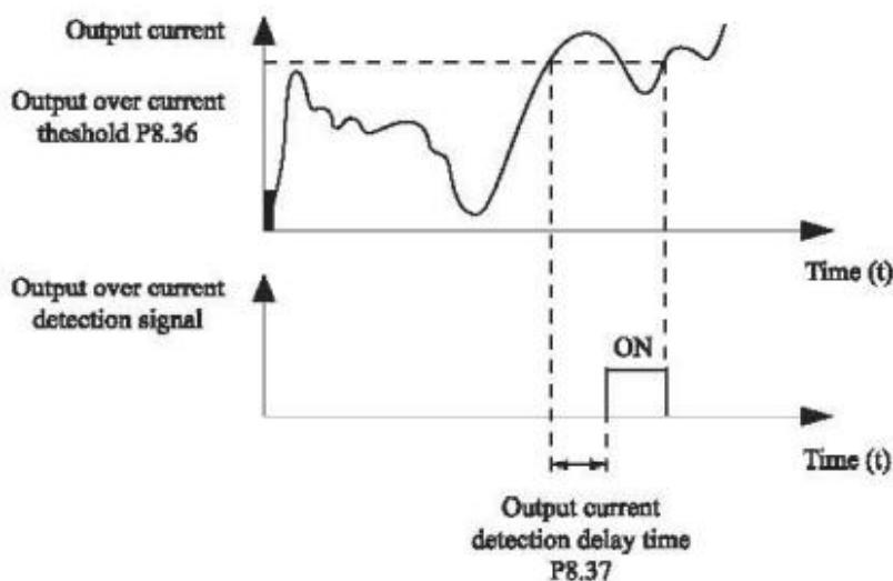
Figure 4-20 Output over current detection
