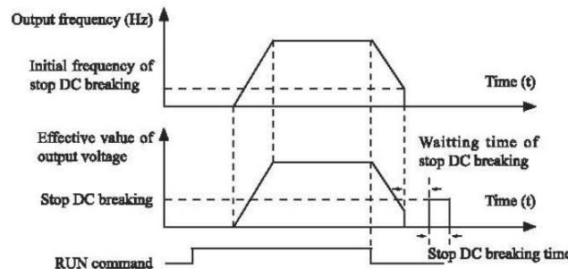
Figure 4-3 Stop DC braking process
