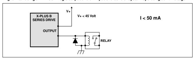
Fig. 7 Driving a micro-relay by means of a X-PLUS B logic output.
