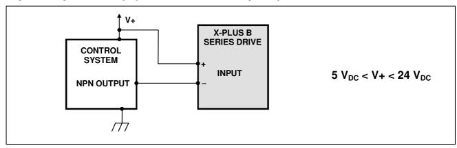
Fig. 8 Driving a X-PLUS B logic input from a control system with a NPN open collector output.
