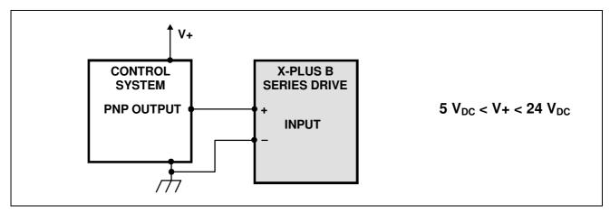
Fig. 9 Driving a X-PLUS B logic input from a control system with a PNP output.
