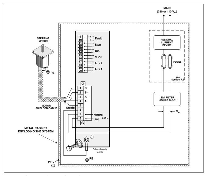
Fig. 5 – Drive external connections scheme.
