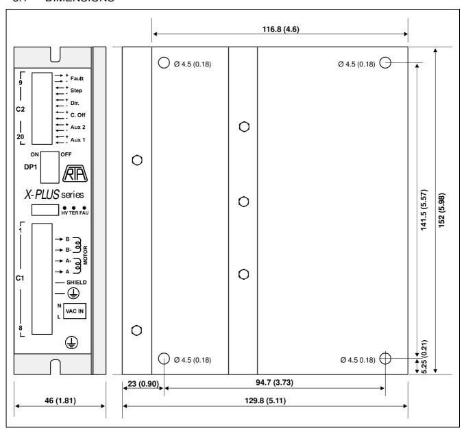
Fig. 2 – Dimensions: all measures in mm.
