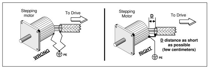
Fig. 1210 Shielded connection at stepping motor side.
