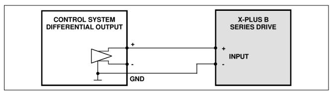
Fig. 11 - Connection example with control system with DIFFERENTIAL output (or LINE DRIVER or RS422).
