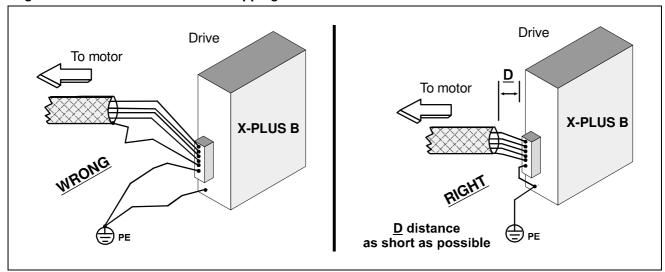
Fig. 13 Shielded connection at drive side.
