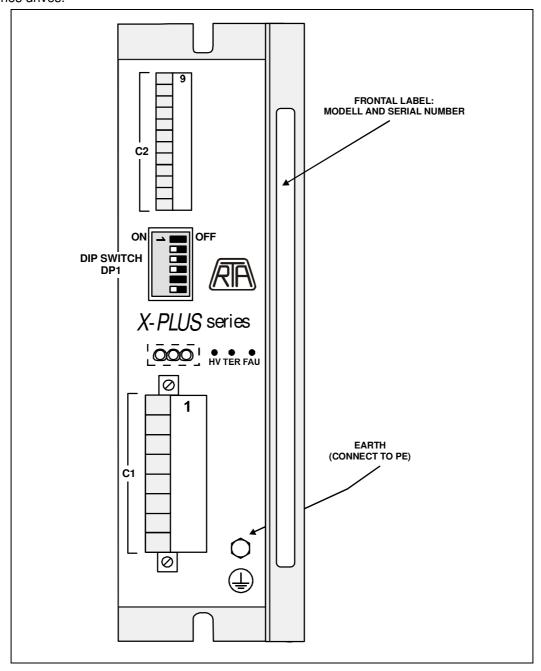
Fig. 4 – Dip-switch DP1, signalling leds and connectors.
