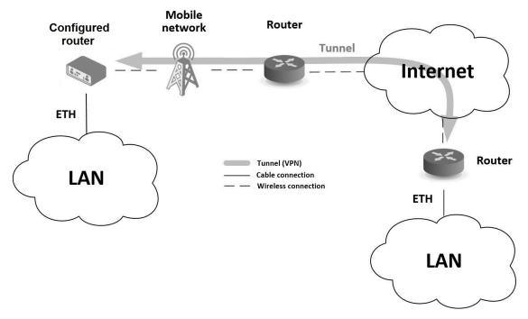
Figure 3: Using VPN Tunnel
