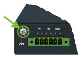
Figure 8: Position of the Grounding Screw
