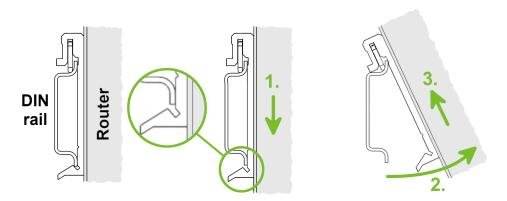
Figure 9: Removing Router from the DIN Rail
