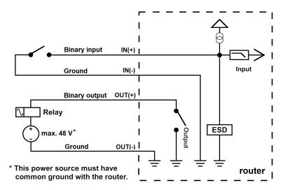
Figure 10: Functional Scheme of the Binary Interface
