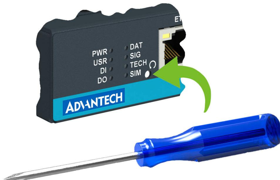
Figure 12: Resetting the Router
