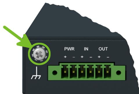
Figure 8: Position of the Grounding Screw
