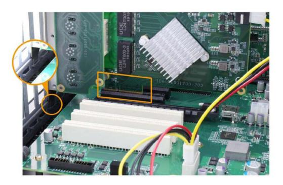
5. Secure the PCIe-PoE312M to finalize the installation.
