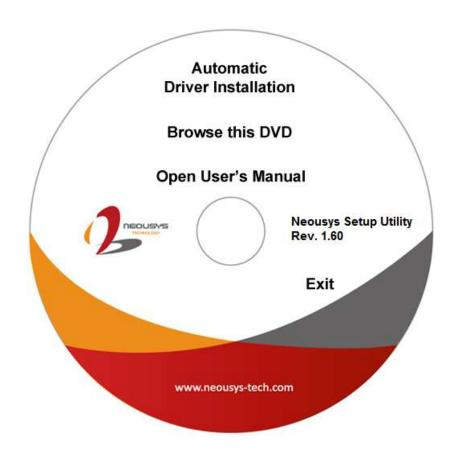
2. Click on the "Automatic Driver Installation". The setup utility will automatically detect your operating system and install corresponding drivers for PCIe-PoE312M. The installation process takes about 2 ~ 3 minutes. Once driver installation is done, the setup utility reboots your Windows and your system works normally afterward.
