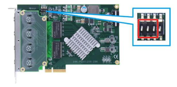
You can configure the board ID by set the position of P1 ~ P3 according to the following table.
