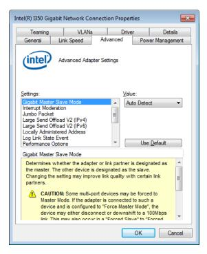
Select the Jumbo Packet settings, and select the expected jumbo frame size. (for connecting a Ethernet device with high data rate, 9014 Bytes is suggested)
