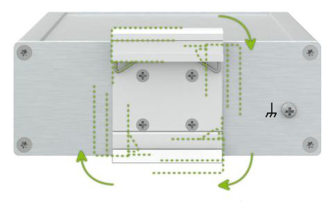
Figure 10: Position of the DIN Rail Clip
