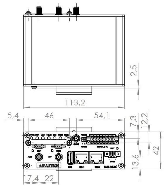
Figure 6: Metal Box - Top and Front View
