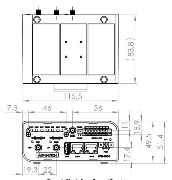
Figure 8: Plastic Box - Top and Front View
