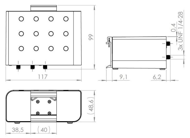
Figure 9: Plastic Box – Bottom, Side and Back View
