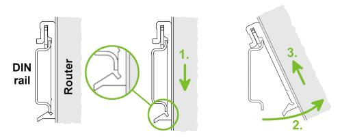
Figure 11: Removing Router from the DIN Rail
