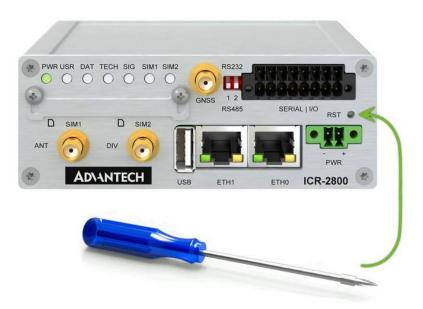
Figure 22: Resetting the Router
