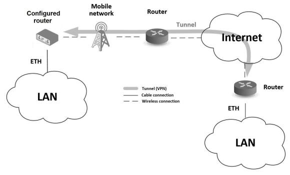
Figure 3: Using VPN Tunnel
