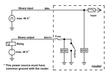
Figure 18: Functional Scheme of the Binary Interface
