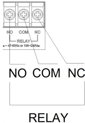
Figure 2.10 Relay output connections
