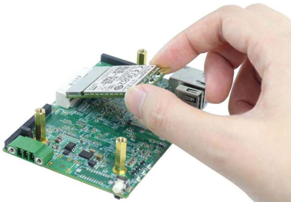
9. Gently press the module down and secure the module with the dedicated screw.
