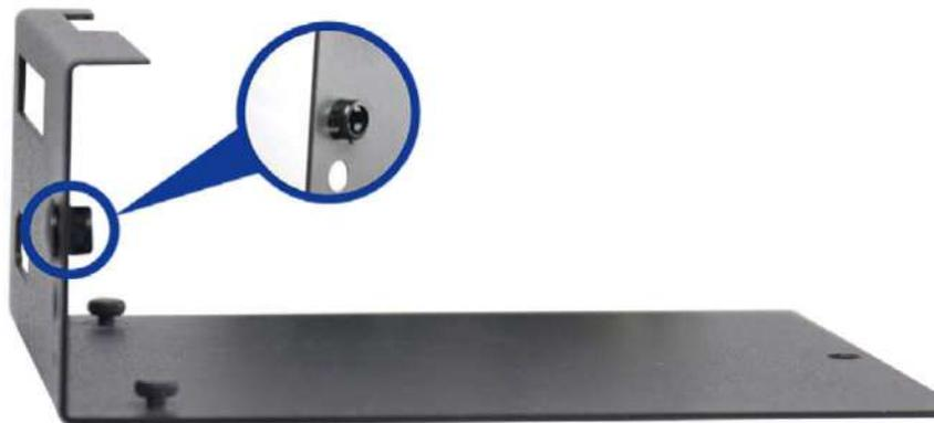
15. To install the SMA female connector, make sure the coupling nut sits outside the enclosure panel, insulator ring sits inside the enclosure panel with the connector body. Fasten the SMA female connector by turning the coupling nut and the connector body in opposite directions. Reinstall the cover and enclosure.
