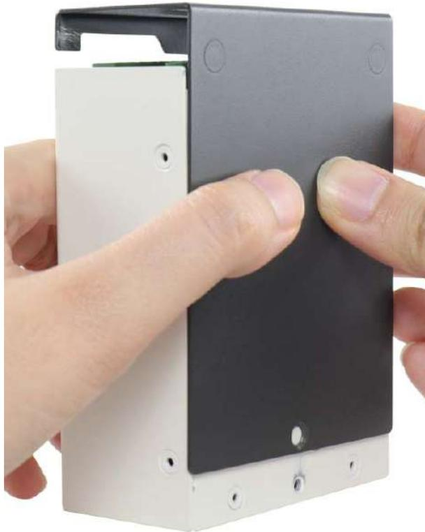
4. Once you have removed the cover, unfasten two screws that secure the PCBA in the enclosure.
