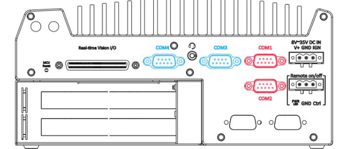
The system provides four COM ports for communicating with external devices. These COM ports are implemented using industrial-grade ITE8786 Super IO chip (-40 to 85°C) and provide up to 115200 bps baud rate.
