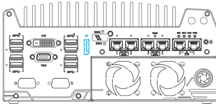
The DisplayPort (DP) is a digital display interface that connects video source and carry audio to a display device. When connecting a DP, it delivers up to 4K UHD (4096 x 2304) in resolution. Designed to support passive DP adapter/ cable, it can connect to other display devices using DP-to-HDMI cable or DP-to-DVI cable.
