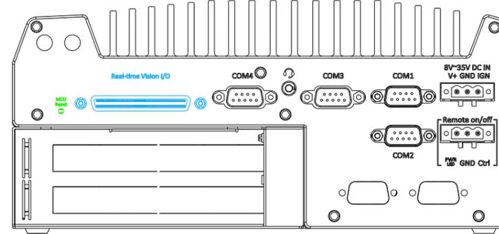
You may use the **MCU reset button** to manually reset the MCU without resetting the whole system. To avoid unexpected resets, the button is purposely placed behind the panel. To reset, please use a pin-like object (eg. tip of a pen) to access the reset button.
