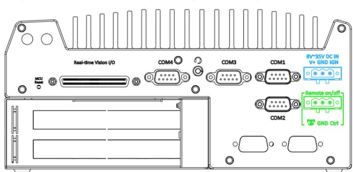
The system accepts a wide range of DC power input from 8 to 35V via a **3-pin pluggable terminal block**, which is fit for field usage where DC power is usually provided. The screw clamping mechanism on the terminal block offers connection reliability when wiring DC power. In addition to DC power input, this terminal block can also accept ignition signal input (IGN) when ignition control module (eg. MezIO-V20-EP) is installed for in-vehicle applications.
