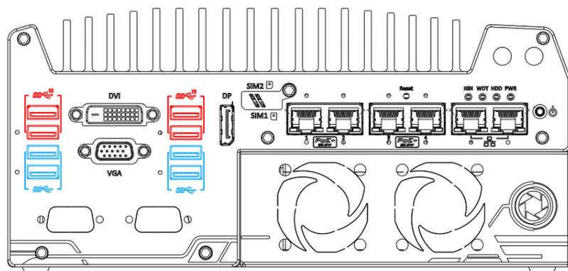
The system's **USB 3.1 Gen 2 (10Gbps)** and **USB3.1 Gen1 (5Gbps)** ports are implemented via native xHCI (eXtensible Host Controller Interface) controller and are backward compatible with USB3.1 Gen.1 USB 2.0, USB 1.1 and USB 1.0 devices. Legacy USB is also supported so you can use USB keyboard/ mouse in DOS environment
