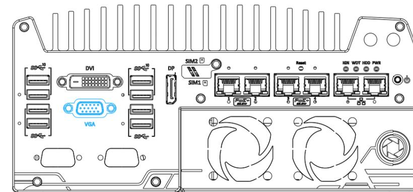
VGA connector is the most common video display connection. The VGA output supports up to 1920x1200@60Hz resolution. The system supports triple independent display outputs by connecting display devices to VGA, DVI and DisplayPort connection. To support multiple display outputs and achieve best VGA output resolution in Windows, you need to install corresponding graphics drivers.
