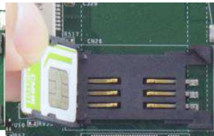
Insert SIM card with pins facing up
