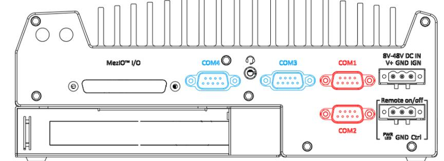
The system provides four COM ports to communicate with external devices. The COM ports are implemented using industrial-grade ITE8786 Super IO chip (-40 to 85°C) and provide up to 115200 bps baud rate. COM1 and COM2 (in red) are software-configurable RS-232/ 422/ 485 ports. COM3 and COM4 (in blue) are standard 9-wire RS-232 ports. The operation mode of COM1 and COM2 can be set in BIOS setup utility. The following table describes the pin definition of COM ports.
