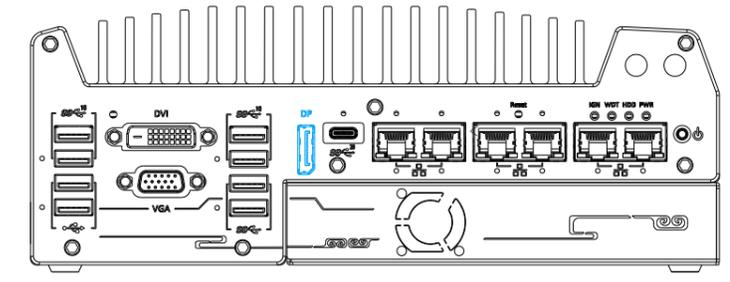
The system has a DisplayPort (DP) output which is a digital display interface that mainly connect video source and carry audio to a display device. When connected to a DP, it can deliver up to 8K UHD (7680 x 4320 @ 60Hz) in resolution. The system is designed to support passive DP adapter/ cable. You can connect to other display devices using DP-to-HDMI cable or DP-to-DVI cable.
