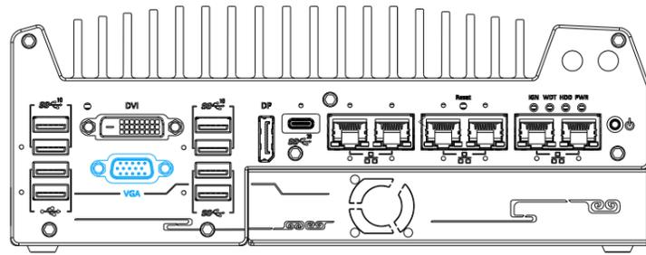
VGA connector is the most common video display connection. The VGA output supports up to 1920x1200@60Hz resolution. The system supports triple independent display outputs by connecting display devices to VGA, DVI and DisplayPort connection. To support multiple display outputs and achieve best VGA output resolution in Windows, you need to install corresponding graphics drivers.
