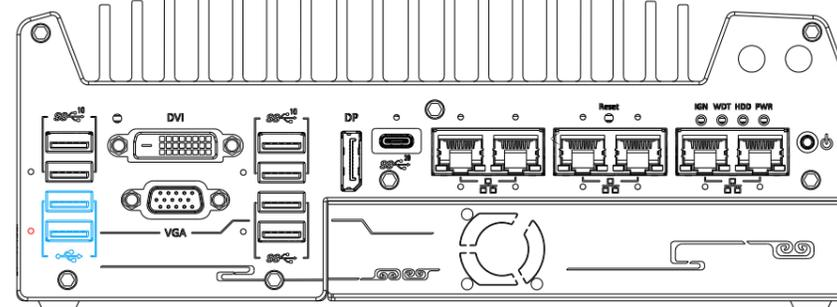
The USB2.0 ports are implemented via native xHCI (eXtensible Host Controller Interface) and are backward compatible with USB 1.1 and USB 1.0 devices. UEFI USB support is also provided so you can use USB keyboard/ mouse in UEFI shell environment. Indicated in **red** is a screw-lock hole for the corresponding USB port. xHCI driver is supported natively in Windows 10, therefore you do not need to install xHCI driver to utilize USB functions.
