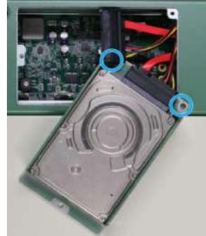
2 screws on each side per HDD/ SSD
