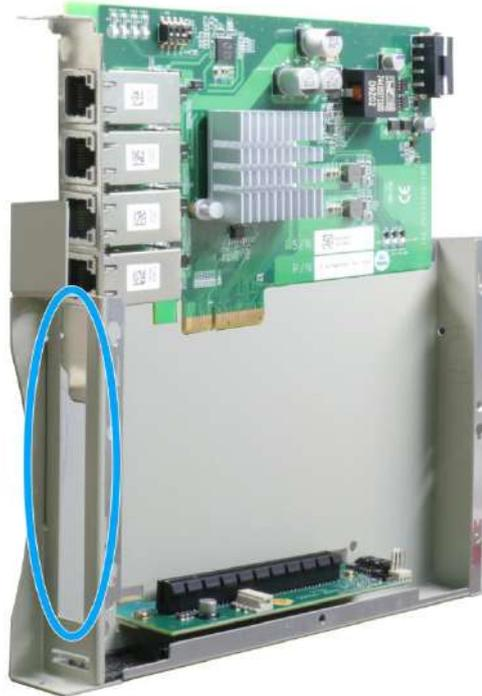
**Remove bezel cover and insert the card**
