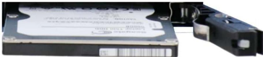
3. Push the handle into the 2.5" slot until it snaps into position. A key is provided (in accessory box) to lock the external slot.
