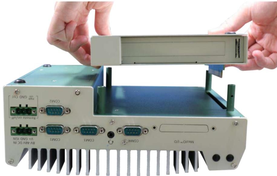
3. Remove the screw to open the Cassette cover.
