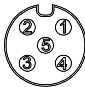
Figure 2.6 Standard M12 5-Pin DC Power Input Connector
