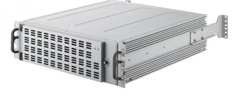
Designed to be both compact, versatile, and powerful, the RMS 400 is a 3U rugged rackmount server with massive storage for extreme versatility. This unit comes with 8 3.5" removable trays and 2 2.5" removable trays. Meeting MIL-STD-810G requirements, this unit can perform under the harshest conditions.
