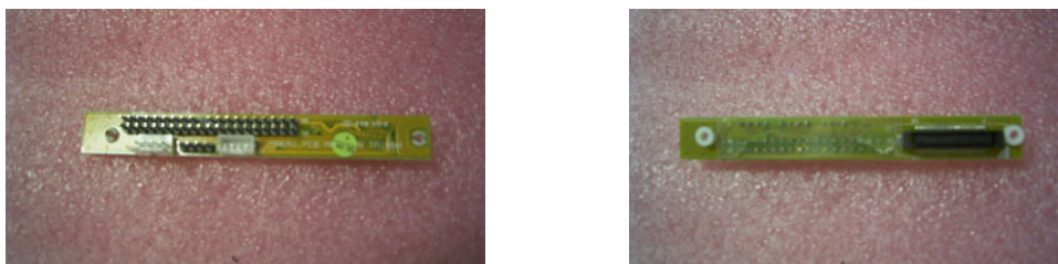
Figure 2.8 Small converter for ATA (IDE) slim-type ODD
