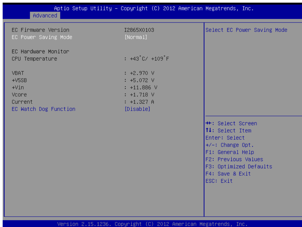
Figure 5.15 Embedded Controller Configuration
