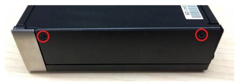
2. Unscrew the 4 screws on the HDD bay.
