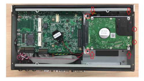
4. Fix the 4 screws back onto the HDD bay.
