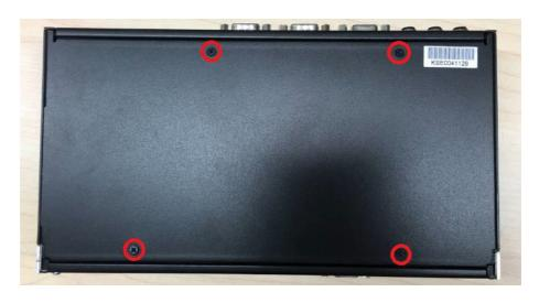
3. Unscrew the 4 screws on the bottom cover and on both sides of ARK-2230.
