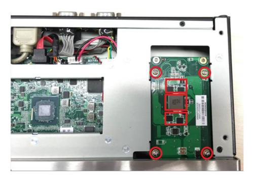
7. Screw the new power bracket for MIOe-PWR2 on the front panel.
