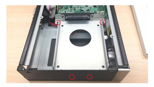
3. Install the HDD/SSD into the HDD bay, and fix the HDD onto the bracket.
