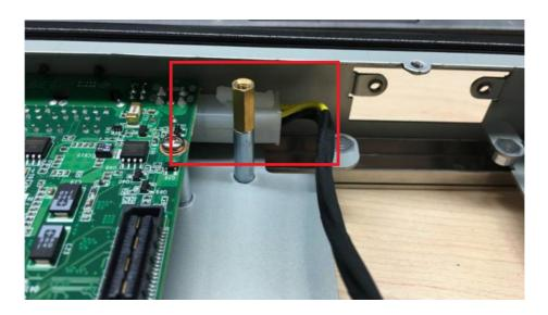
5. Link the MIOe-PWR2 internal power cable from M/B to the power board.
