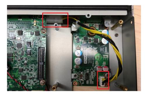
6. Turn to the top side, and fasten the 4 screws for the power board, and tape 3 thermal pads on the red marks.
