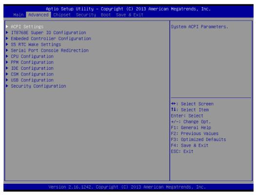
Figure 3.3 Advanced BIOS features setup screen
