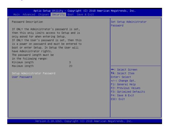
Select Security Setup from the ARK-2232 Setup main BIOS setup menu. All Security Setup options, such as password protection and virus protection are described in this section. To access the sub menu for the following items, select the item and press <Enter>:
