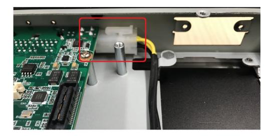
5. Link the MIOe-PWR2 internal power cable from M/B to the power board.
