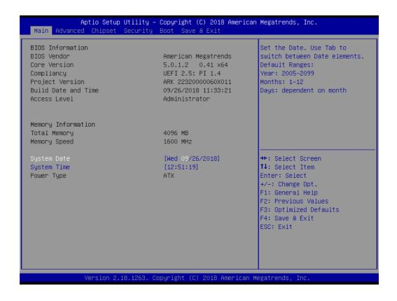
AMI BIOS ROM has a built-in Setup program that allows users to modify the basic system configuration. This information is stored in battery-backed CMOS so it retains the Setup information when the power is turned off.
