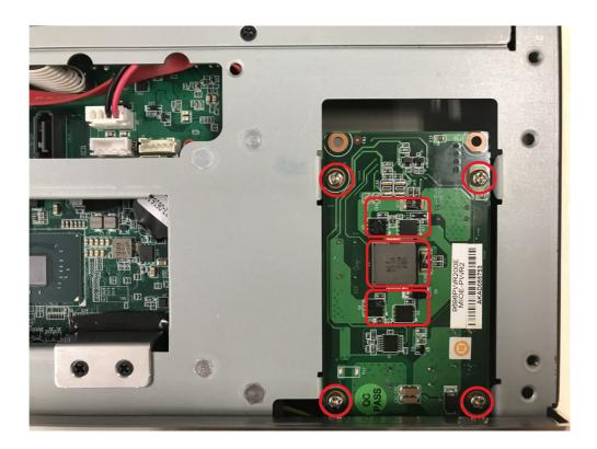
7. Screw the new power bracket for MIOe-PWR2 on the front panel.
