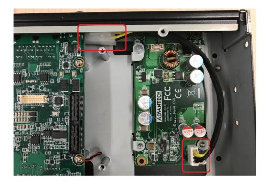
6. Turn to the top side, and fasten the 4 screws for the power board, and tape 3 thermal pads on the red marks.
