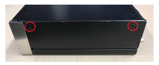
2. Unscrew the 4 screws on the HDD bay.
