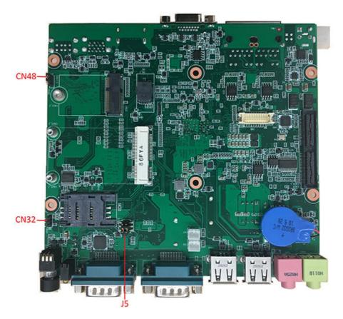
Figure 2.1 Jumper Layout
