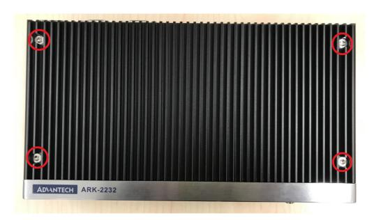
2. Remove the top cover and install the memory into the memory socket.
