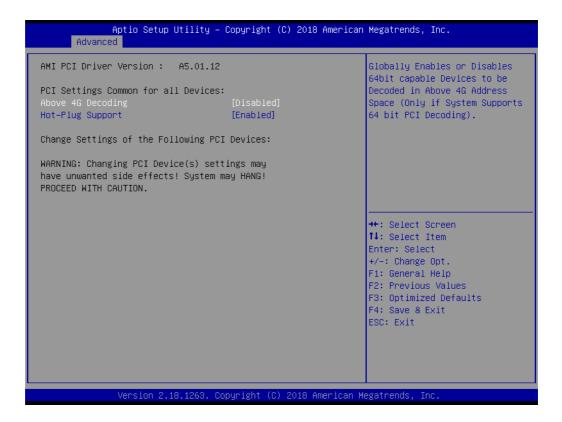
Above 4G Decoding Enable or Disable Above 4G Decoding device.
