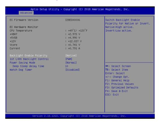
Embedded controller configuration displays all information about system Temperature/Voltage.
