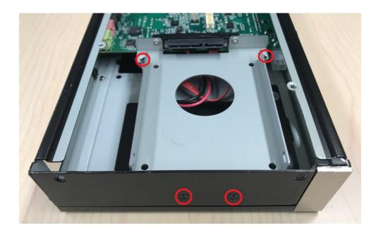
3. Install the HDD/SSD into the HDD bay, and fix the HDD onto the bracket.
