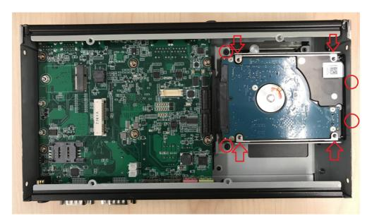
4. Fix the 4 screws back onto the HDD bay.
