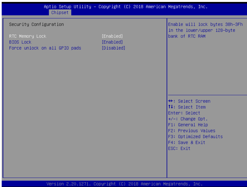
Figure 3.26 Security Configuration Screen
