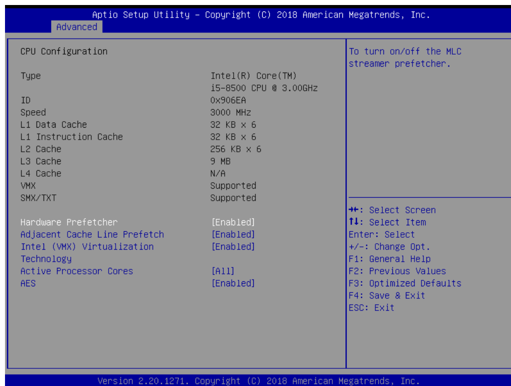
Figure 3.5 CPU Configuration Screen
