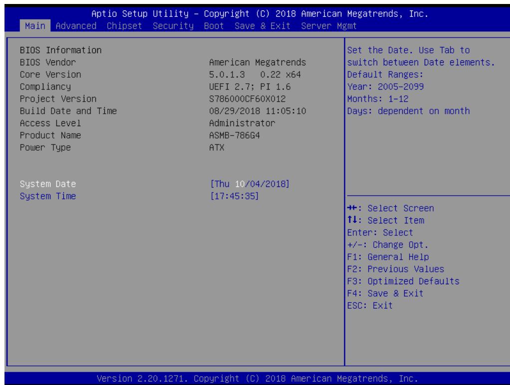
Figure 3.1 Main BIOS Setup Screen
