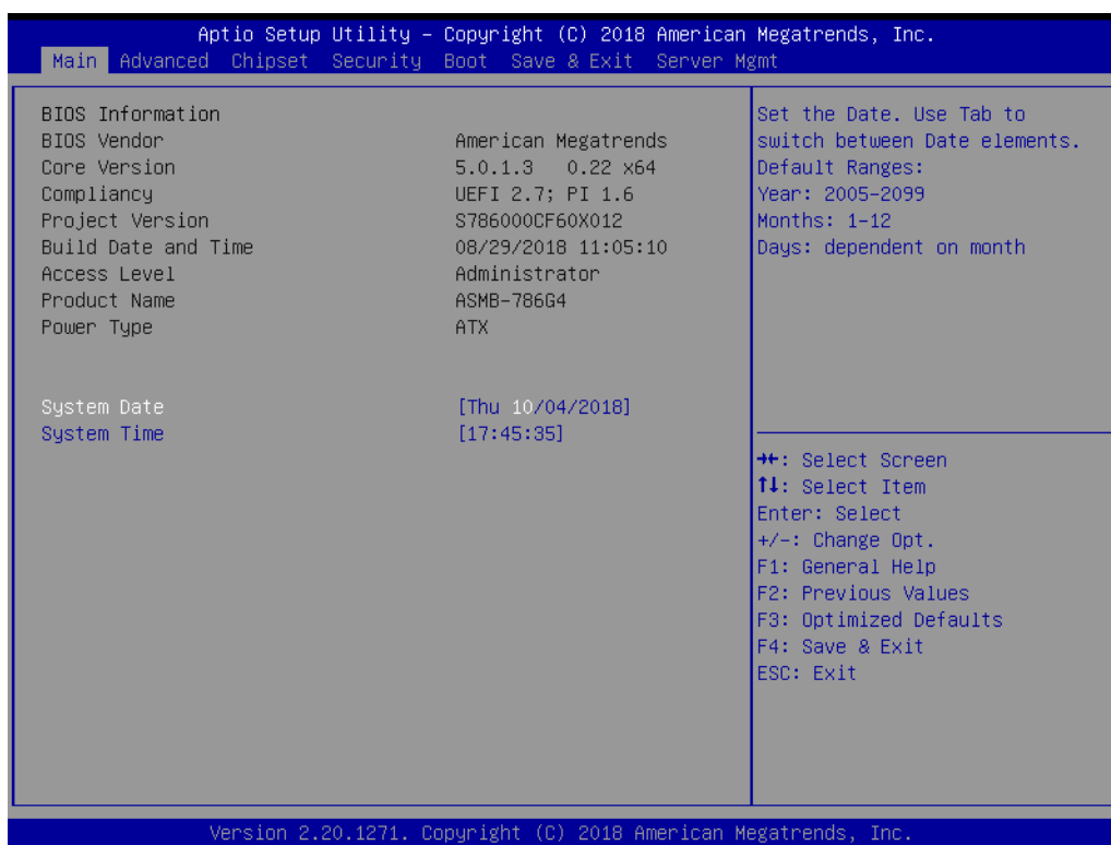
Figure 3.2 Main BIOS Setup Screen
