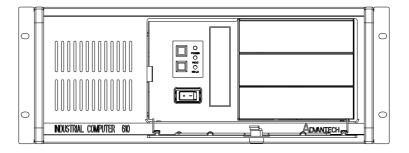
Figure 3.1 Front panel of IPC-610-F
