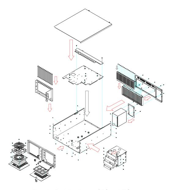
Figure A.5 Exploded diagram of IPC-610-L/IPC-611
