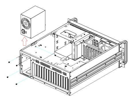
Figure 3.10 Replacing the single power supply
