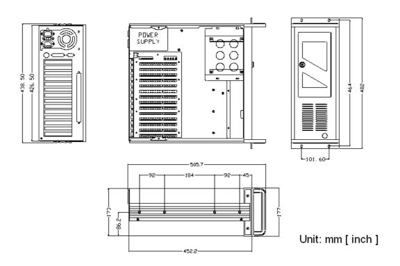
Figure 1.4 Dimension diagram of IPC-610-E
