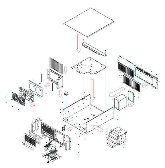
Figure A.2 Exploded diagram of IPC-610-H
