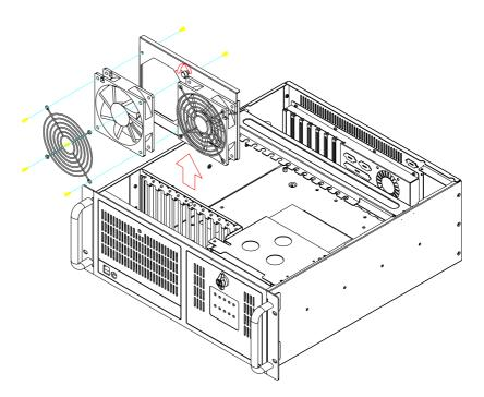
Figure 3.4 Replacing the cooling fan for ACP-4000/IPC-610-H
