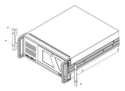
Figure 2.8 Attaching the ears and handles
