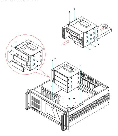
Figure 2.7 Installing disk drives
