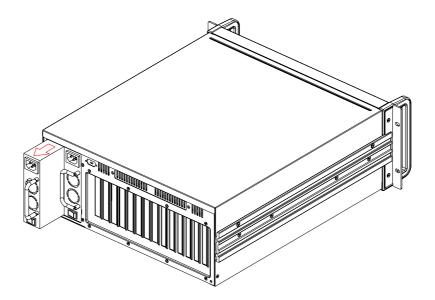
Figure 3.11 Replacing the power supply module
