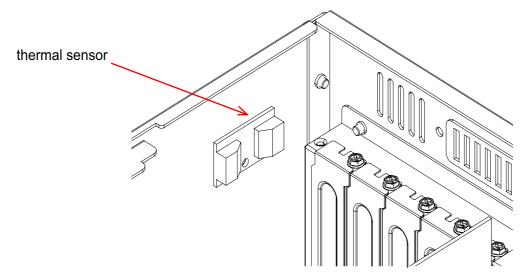
Figure 4.2 Thermal sensor location
