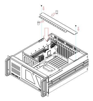
Figure 2.6 Installing rubber cushions and hold-down clamp
