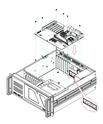
Figure 2.4 Installing a motherboard
