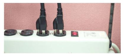
Figure 3.12 Power cord plugs orientation on the socket
