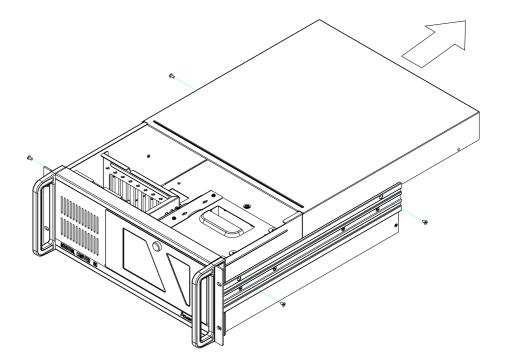
Figure 2.1 Removing the top cover
