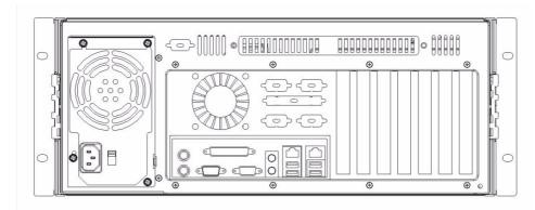
Figure 3.3 Rear panel of motherboard version
