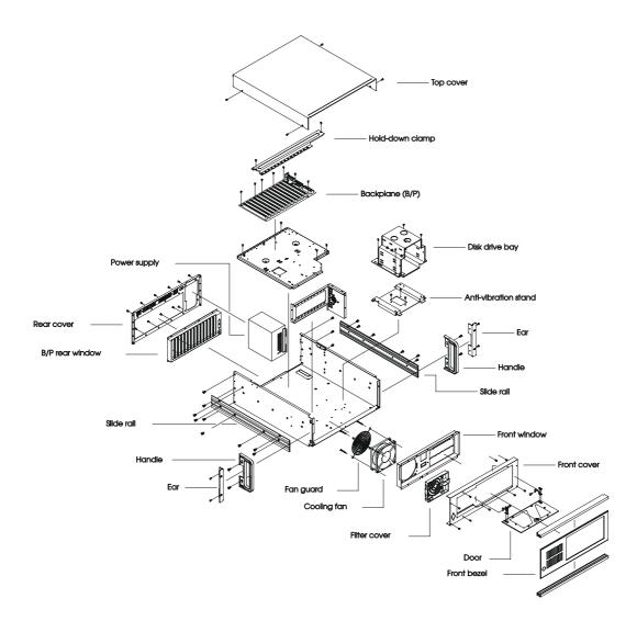
Figure A.4 Exploded diagram of IPC-610-E
