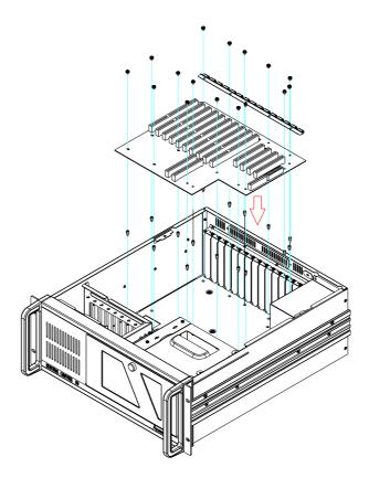
Figure 2.3 Installing the backplane
