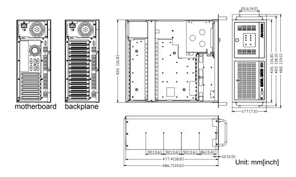
Figure 1.2 Dimension diagram of IPC-610-H
