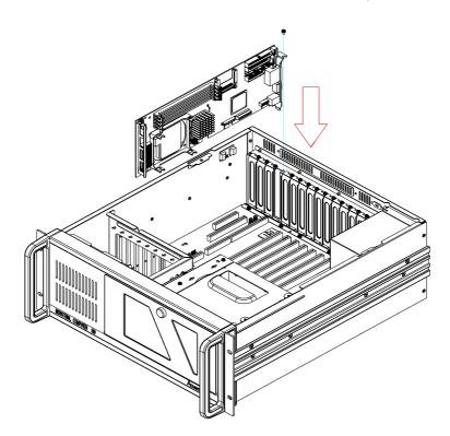
Figure 2.5 Installing a full-length card
