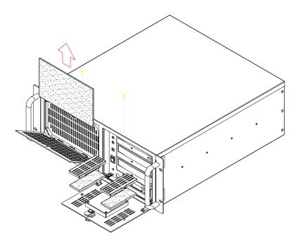
Figure 3.7 Replacing the filters for ACP-4000/IPC-610-H
