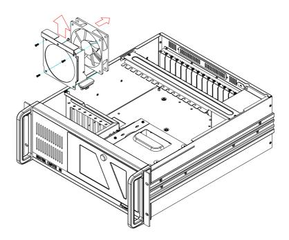
Figure 3.5 Replacing the cooling fan for IPC-610-F
