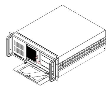
Figure 3.8 Replacing the filters for IPC-610-F/IPC-610-E
