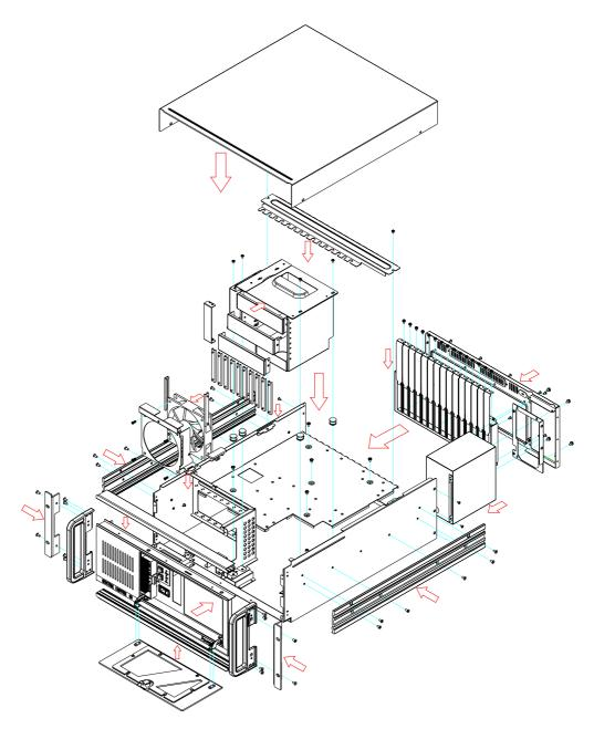
Figure A.3 Exploded diagram of IPC-610-F
