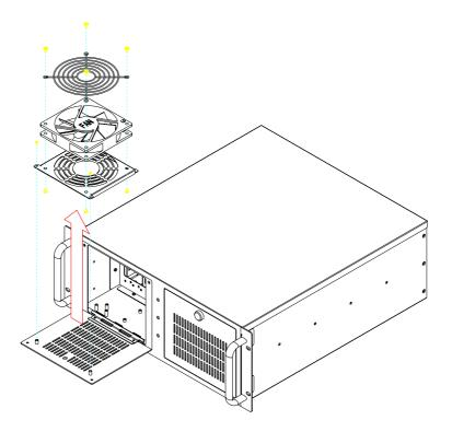
Figure 3.6 Replacing the cooling fan for IPC-610-L/IPC-611
