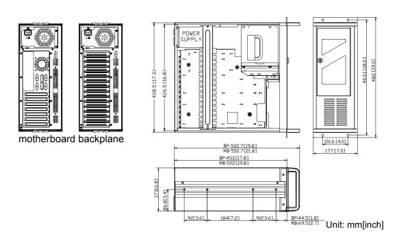
Figure 1.3 Dimension diagram of IPC-610-F
