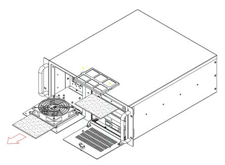
Figure 3.9 Replacing the filters for IPC-610-L/IPC-611
