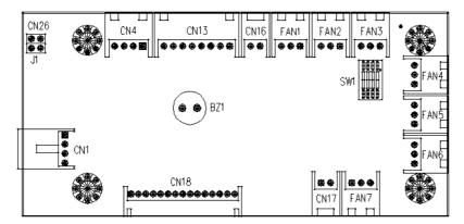
Figure 4.1 Alarm Board Layout
