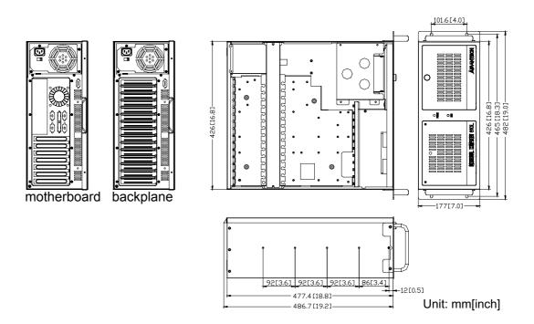
Figure 1.5 Dimension diagram of IPC-610-L
