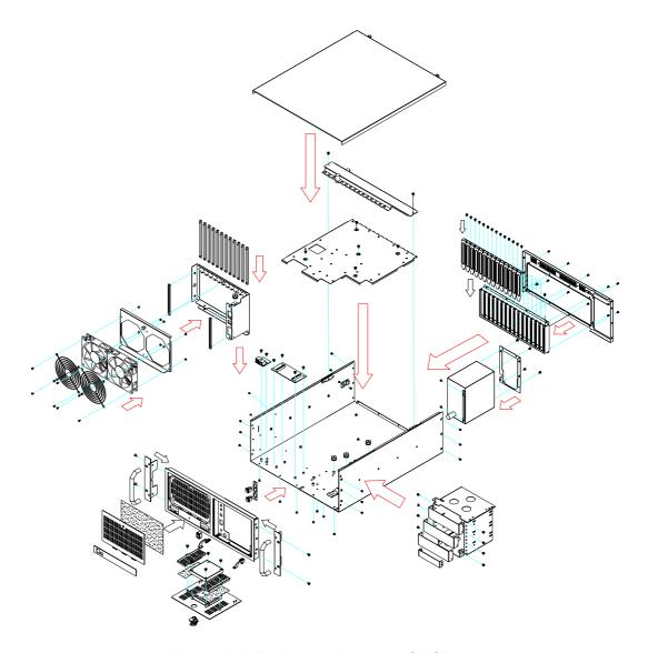
Figure A.1 Exploded diagram of ACP-4000
