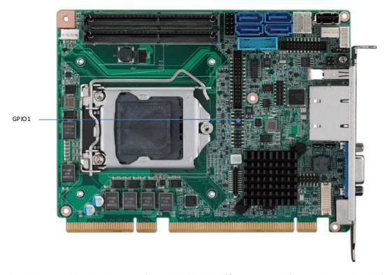
Provides 10-Pin pin header for 8-bit Digital I/O usage. Refer to Appendix B for detailed information on the pin assignments and programming guide in Appendix C.
