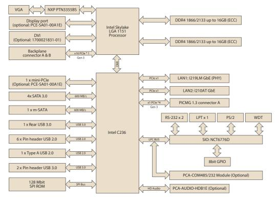
Figure 1.3 PCE-4129 Block Diagram
