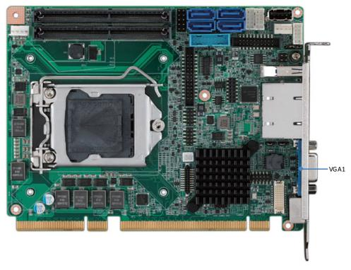
This CPU card has VGA outputs that can drive conventional CRT displays. VGA1 is a standard 15-pin D-SUB connector commonly used for VGA.
