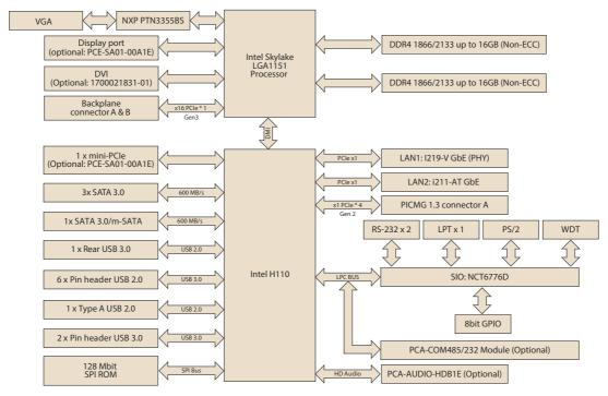
Figure 1.2 PCE-3029 Block Diagram
