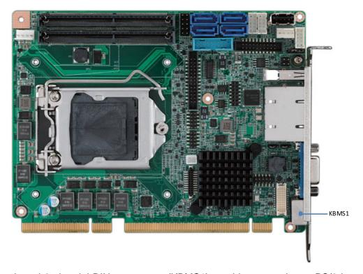
Two on-board 6-pin mini-DIN connectors (KBMS1) provide connection to PS/2 keyboard.
