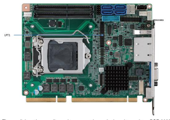
The parallel port is normally used to connect the motherboard to a printer. PCE-3029/4129 includes an onboard parallel port, accessed through a 26-pin flat-cable connector, LPT1.
