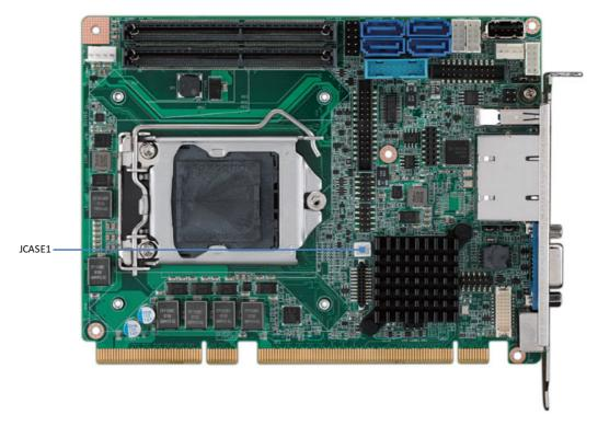
The 2-pin case open connector is for chassis with a case open sensor. When the case is open, the buzzer on motherboard will beep.
