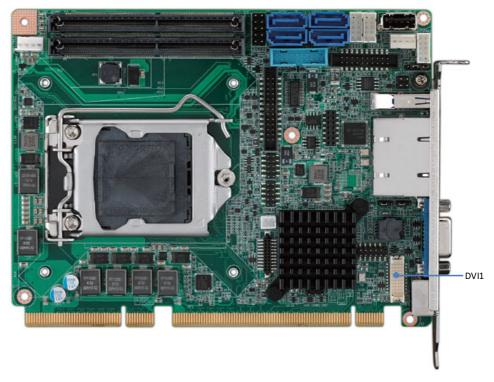
DVI1 is a 20-pin connector, supporting resolution up to 1920 x 1200. Please place order no. 1700021831-01 for standard DVI connector on bracket.
