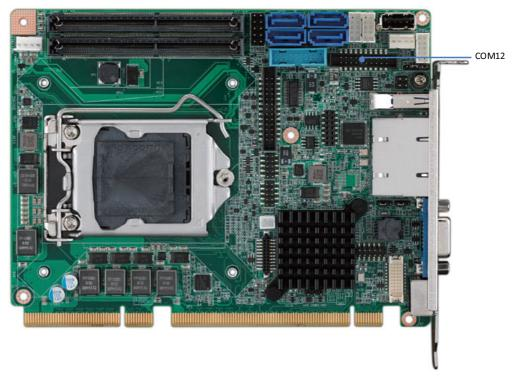
PCE-3029/4129 offers two serial ports. These ports can connect to serial devices, such as a mouse or a printer, or to a communications network. The IRQ and address ranges for both ports are fixed. However, if you want to disable the port or change these parameters later, you can do this in the system BIOS setup.
