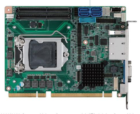
PCE-3029/4129 features high performance serial ATA 3.0 interface which eases cabling to hard drivers or CD/DVD drivers with long cables.
