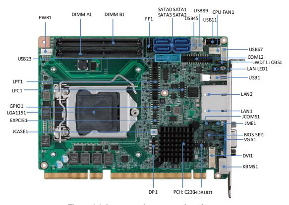
Figure 1.1 Jumper and connector locations
