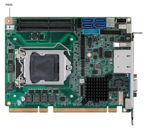
Due to no 5V supply from the golden fingers, please use a power converter: 1703040100 to connect from the peripheral power connector on the power supply to PWR1 on board.
