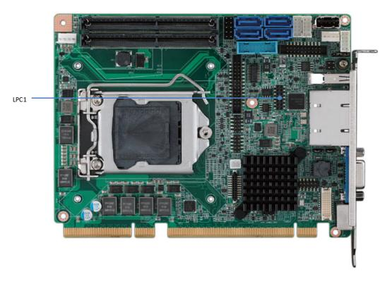
LPC1 is a 14-pin female pinheader for adopting Advantech LPC module, such as PCA-COM232-00A1E, PCA-COM485-00A1E, PCA-TPM-00A1E.
