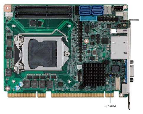
This HDAUD1 pin header is the connection interface to Advantech's audio module.
