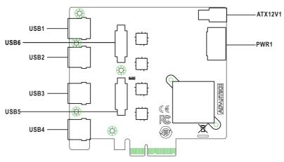
Figure 1: Main Board Connectors Locations
