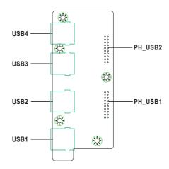
Figure 2: USB Carrier Board Connectors Locations
