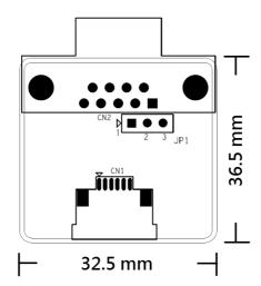
Figure 4.1 CAN-bus transceiver board silk screen
