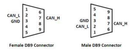
Figure 4.3 PCM-26D2CA DB-9 connector pin assignments
