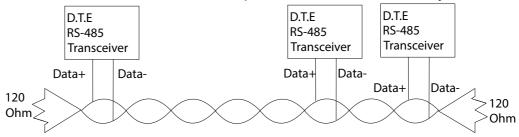
Figure 3.1 RS-485 Wiring Topology
