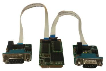
Figure 4.5 FPC cable wiring
