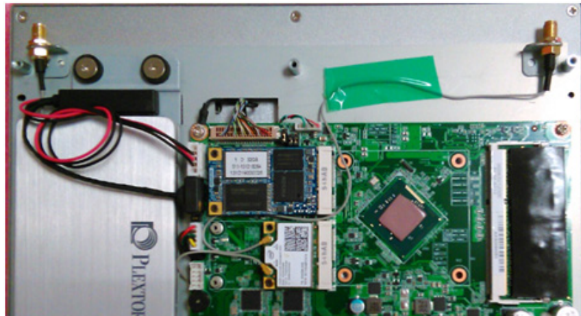
Figure 2.18 Half-size mini PCIe LAN antenna cables
