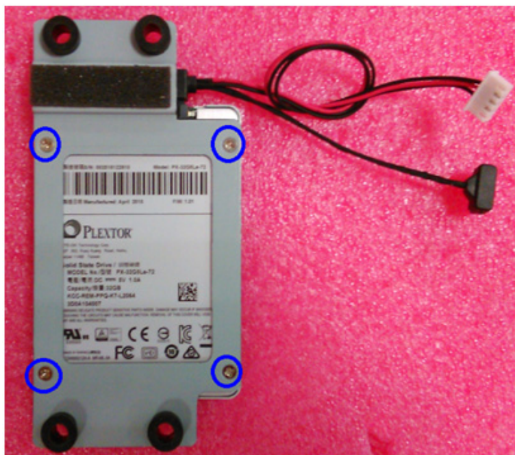
Figure 2.11 Secure SATA HDD with screws
