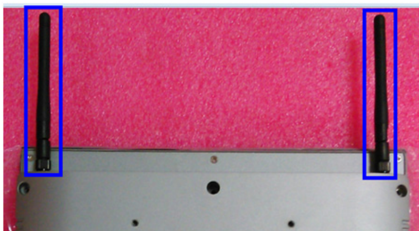
Figure 2.21 Location of external antennae
