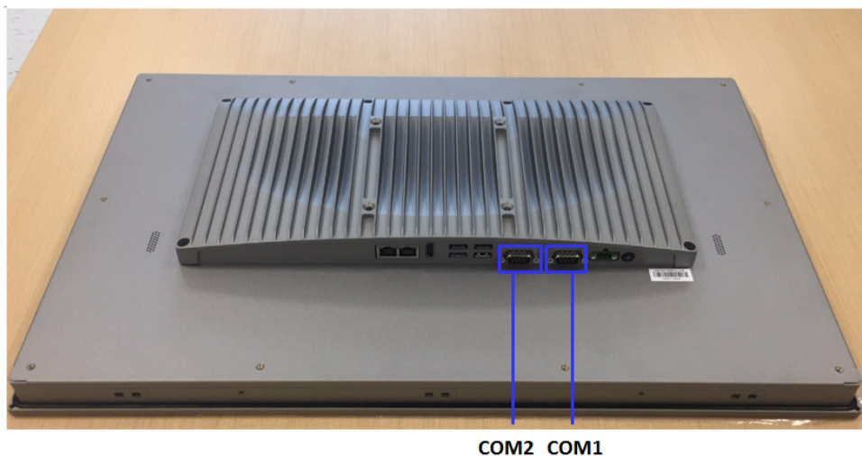
Figure 3.3 Location of COM1 and COM2 ports
