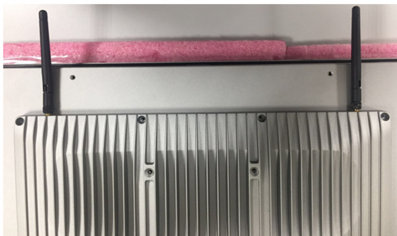
Figure 2.17 Location of external antennae
