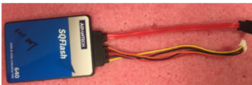
Figure 2.9 SATA cable connected to SATA HDD
