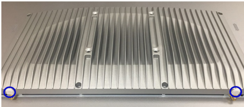
Figure 2.16 Removing plugs for the antennae
