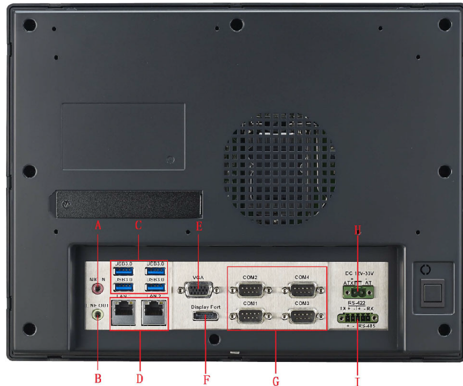
Figure 2.3 IO Connectors of Panel PC
