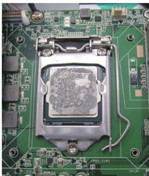
Figure 2.8 CPU fasten in socket
