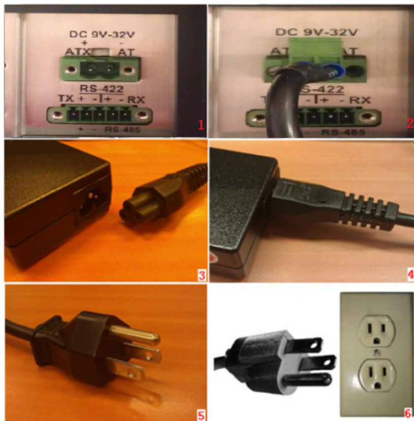
Figure 2.4 Connecting Power Cord
