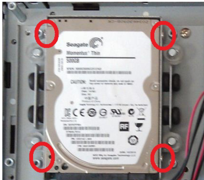
Figure 2.13 Fix HDD in HDD brackets
