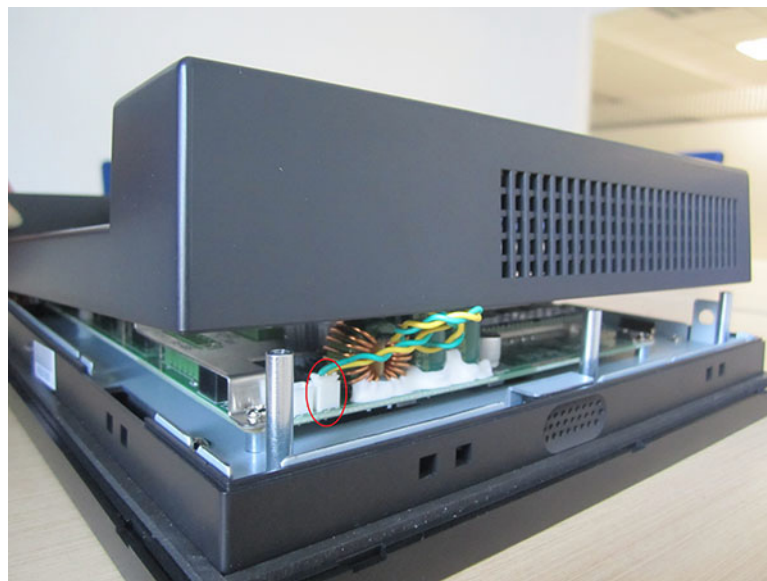
Figure 2.6 Unplugging Switch Wire
