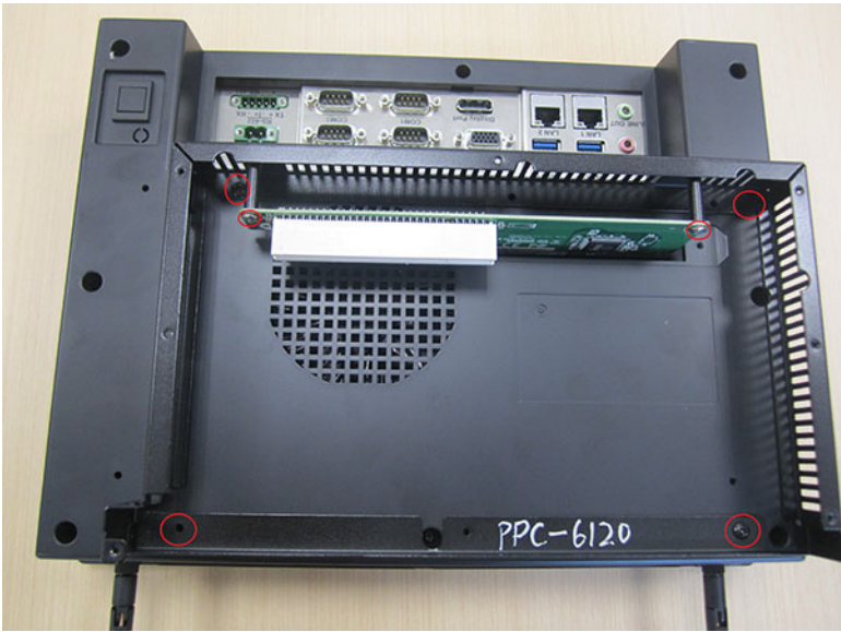
Figure 2.21 Assemble riser card
