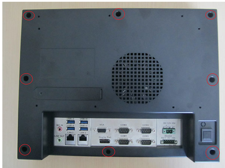
Figure 2.5 Unfastening Screws on Rear Cover
