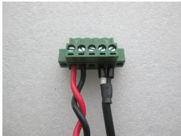
**Figure 2.8 Positive and negative cables**
