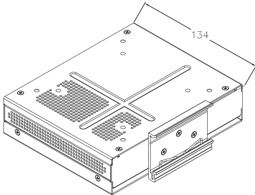
**Figure 1.3 Install with din-rail bracket**
