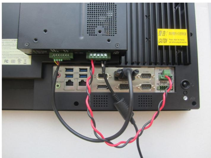
**Figure 2.19 Connecting the power and control cables**
