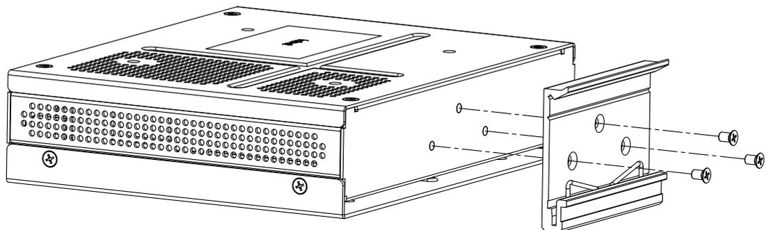
Figure 2.4 DIN Rail Mounting
