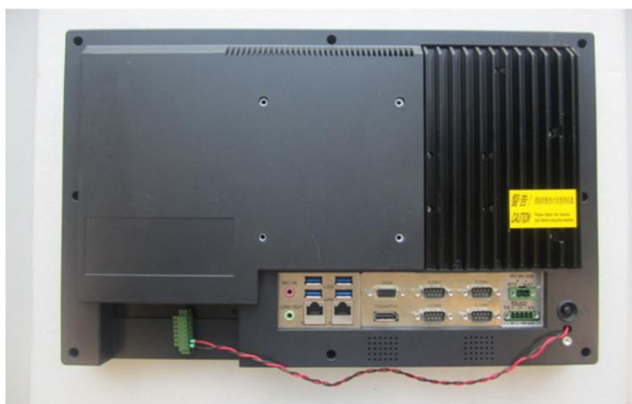
**Figure 2.15 Finished power cable**
