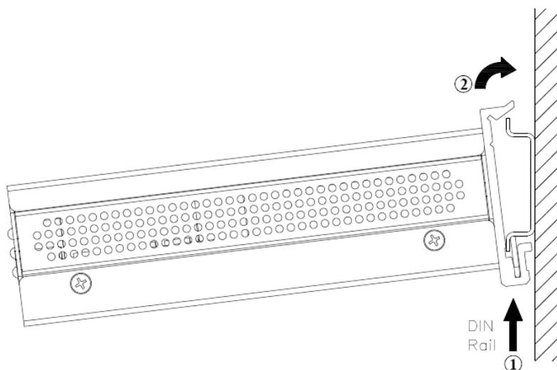
**Figure 2.5 Attaching the IPS to a DIN Rail**
