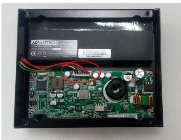
Figure 2.25 Open IPS Power connector position
