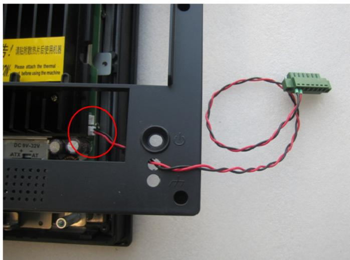
**Figure 2.14 Feeding the cable through the punch hole**
