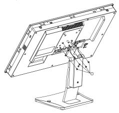
**Step 4**: As the figure below shows, use  $1 \times No. C$  screw in the pack list to secure the hinge cover.
