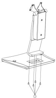
**Step 3**: As the figure below shows use 4 screws of No. B in the pack list to secure the VESA Bracket.
