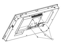
**Step 2**: As the figure below shows, use 4 screws of No. A in pack list to lock on the base plate.
