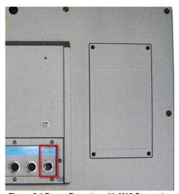
Figure 2.4 Power Receptor with M12 Connector
