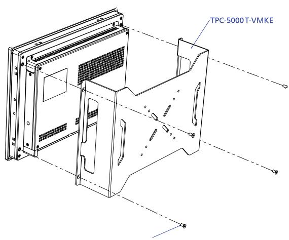
4-M4x8L Screws For FPM-D12T/D15T/D17T/D15W/D18W/D21W/D24W
