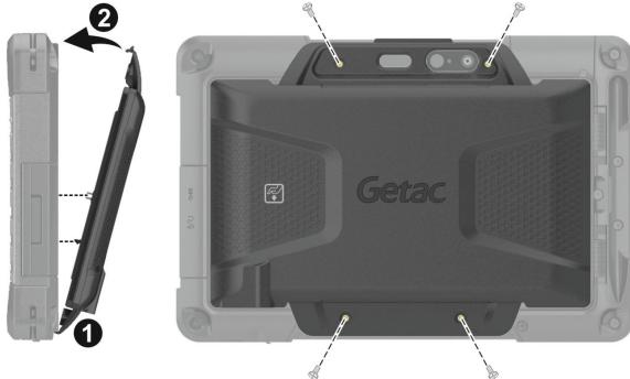
4. When connected, the second battery will be discharged first and then the main battery.
