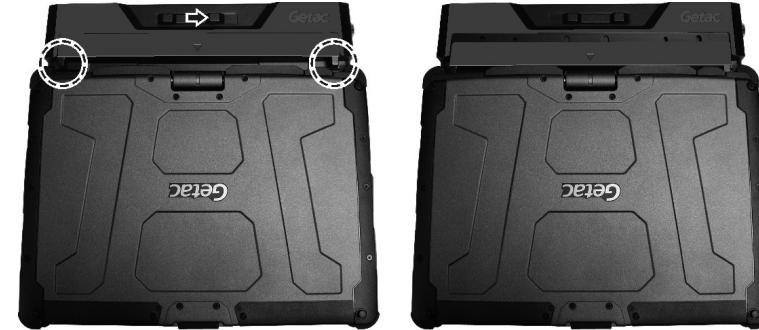
3. Insert the key to the key lock. Press and then turn the lock to the locked position.
