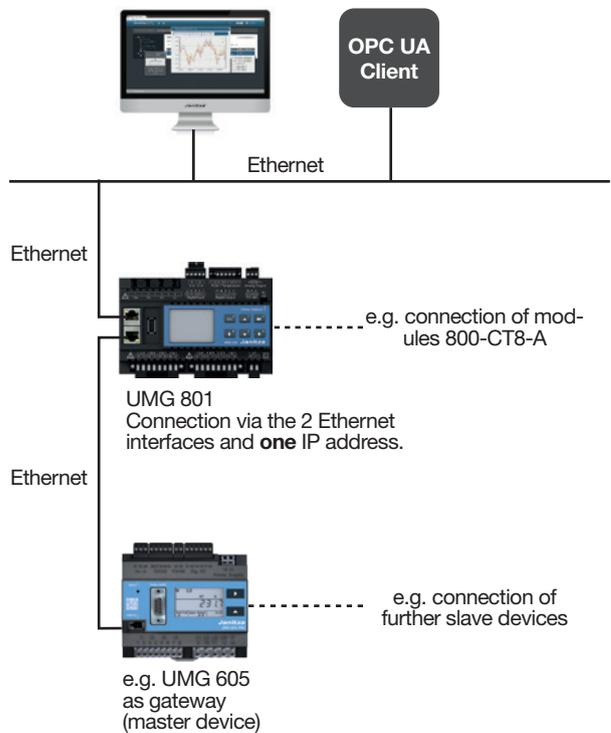
Fig.: UMG 801 in a daisy chain connection
