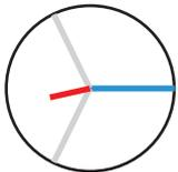
Voltage and current have a deviation of about 180° in the phase position.
