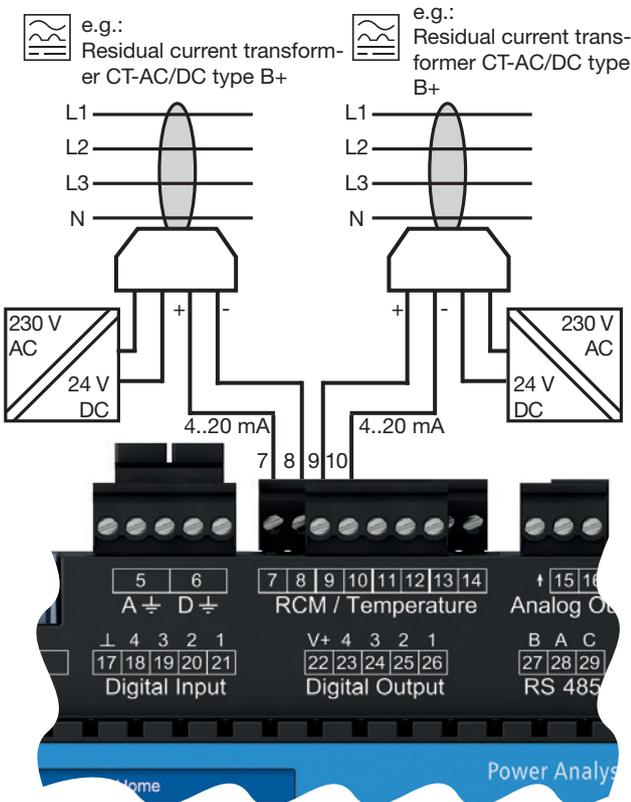
Fig. Connection variant, residual current monitoring via current transformer of Type B. Each residual current transformer of the series CT-AC/DC type B+ RCM requires its own power supply (with  $U = 24\text{ V DC}$ , residual ripple  $< 5\%$ , power =  $24\text{ W}$ ).
