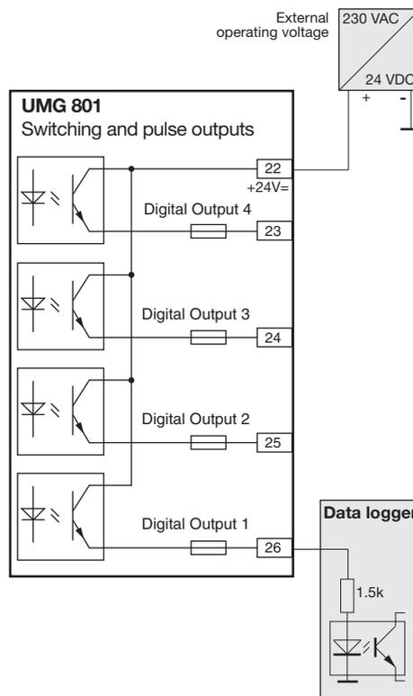
Abb. Connection example for wiring as a pulse output.
