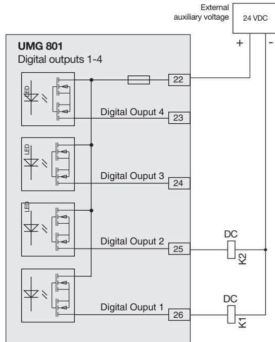
Abb. Connection example of two relays to the digital outputs
