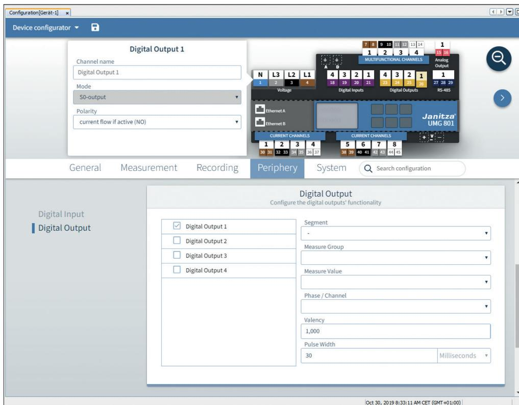
Abb. Assistant for configuring the digital outputs (GridVis® software)
