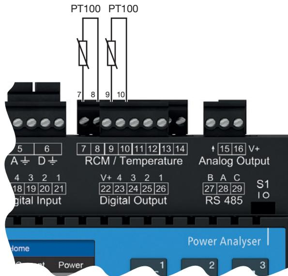
Fig. Connection example "2x temperature measurement" via PT100.
