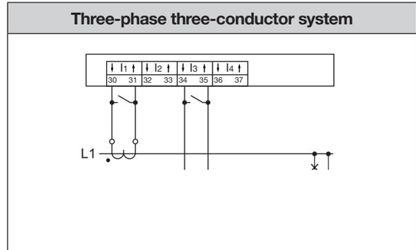
Current measurement via 2 current transformers (Aron circuit)
