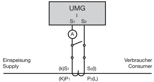
Fig. Example circuit diagram with ammeter in series connection
