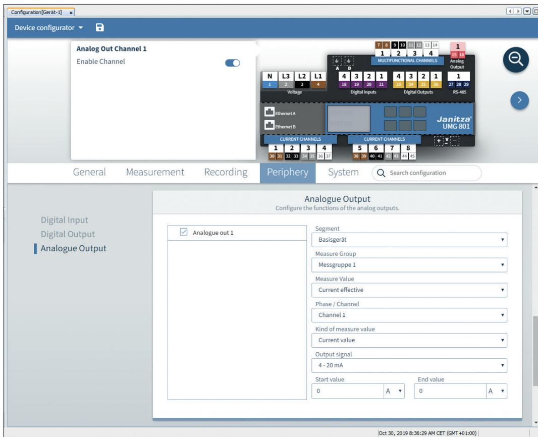
Abb. Assistant for configuration of the analog output (GridVis® software)
