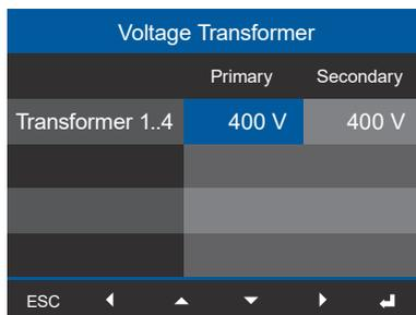
Fig. Window Voltage transformer -> item Primary for voltage transformer 1..4.
