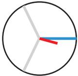
Voltage and current have only a small deviation in the phase position.
