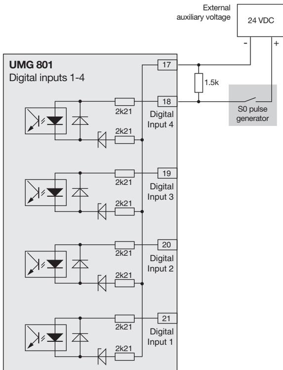
Abb. Example for the connection of an S0 pulse generator to digital input 1.
