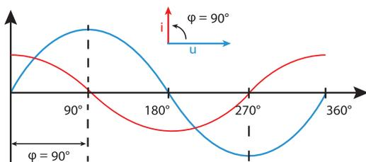
With a combination of the states, the phase angle "current to voltage" can assume values between  $-90^\circ$  and  $+90^\circ$ .
