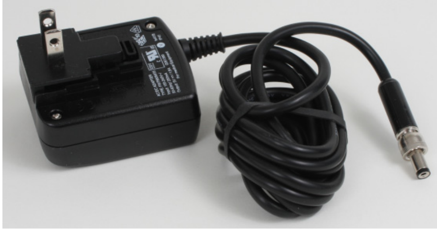
Figure 6: EP394 External +5 V Power Supply
