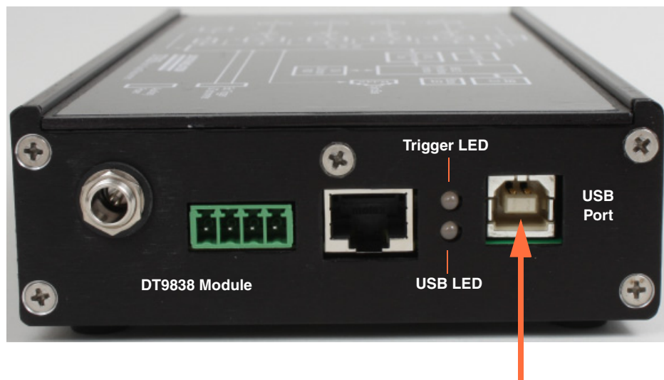
Figure 10: Attaching the DT9838 Module to the Host Computer
