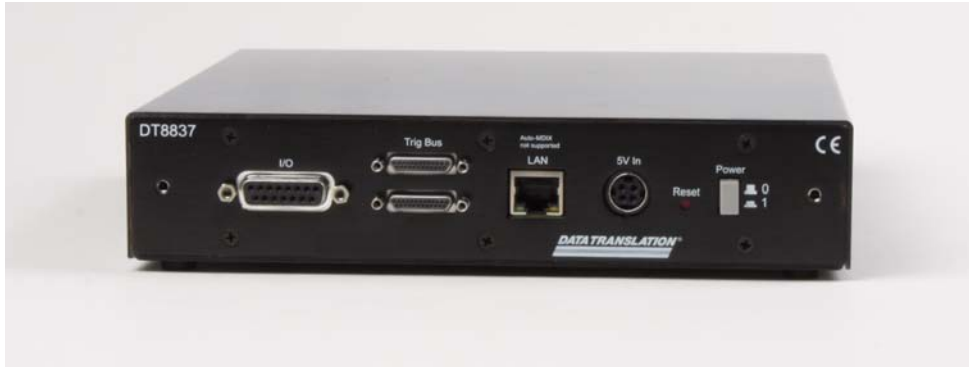
Figure 8: Rear Panel of the DT8837
