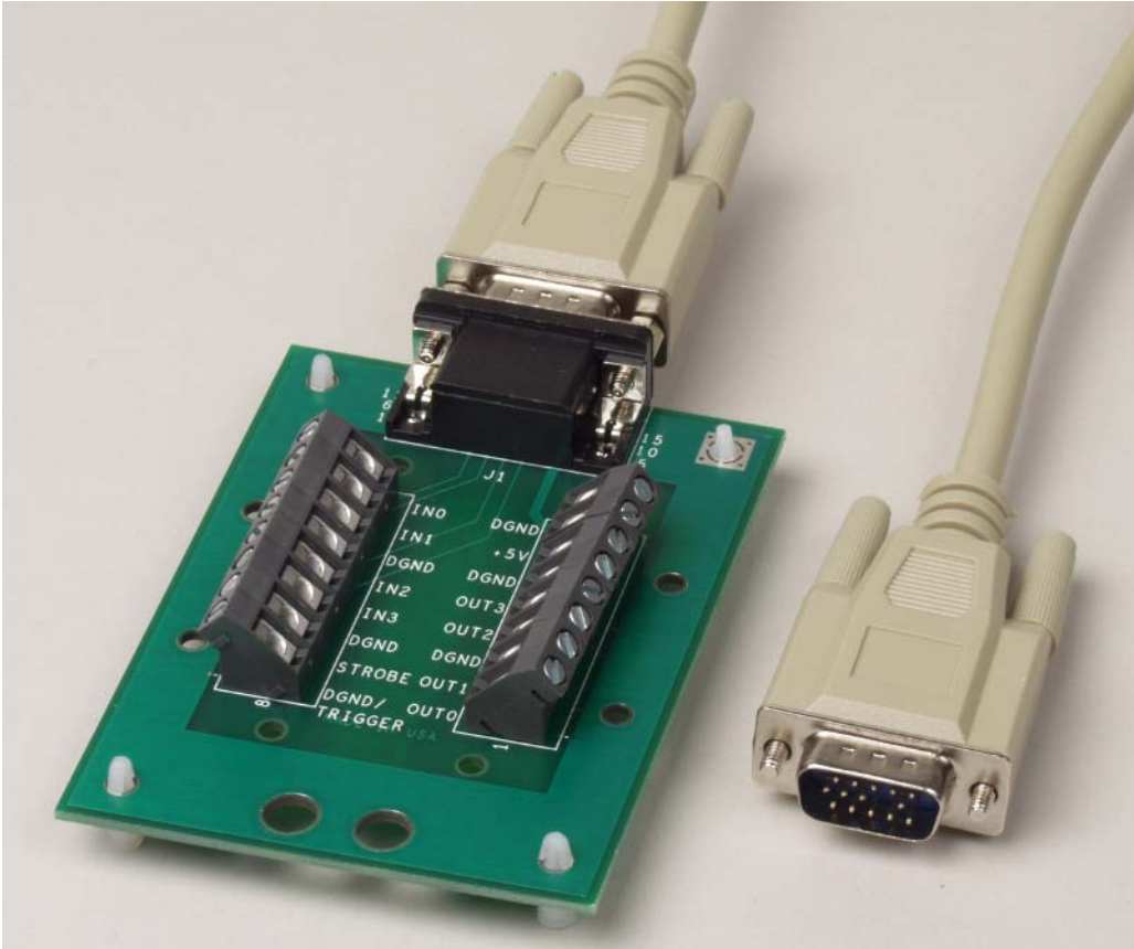
Figure 2: STP15 Screw Terminal Panel and EP337 Cable
