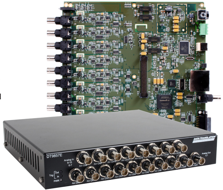
Figure 1. The DT9857E offers many capabilities for vibration measurement such as 16 IEPE 24-bit Delta-Sigma sensor inputs, two 32-bit D/A stimulus outputs, a 32-bit tachometer, pre- and post-triggering. The Sync Bus allows expansion to 64 analog input channels and 8 analog output channels, and the ability to time sync all data to the input data stream.
