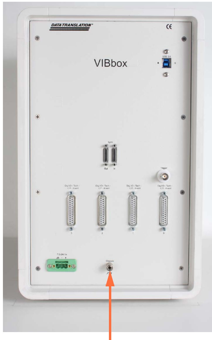
Connect Grounding Strap to the Chassis Grounding Stud
