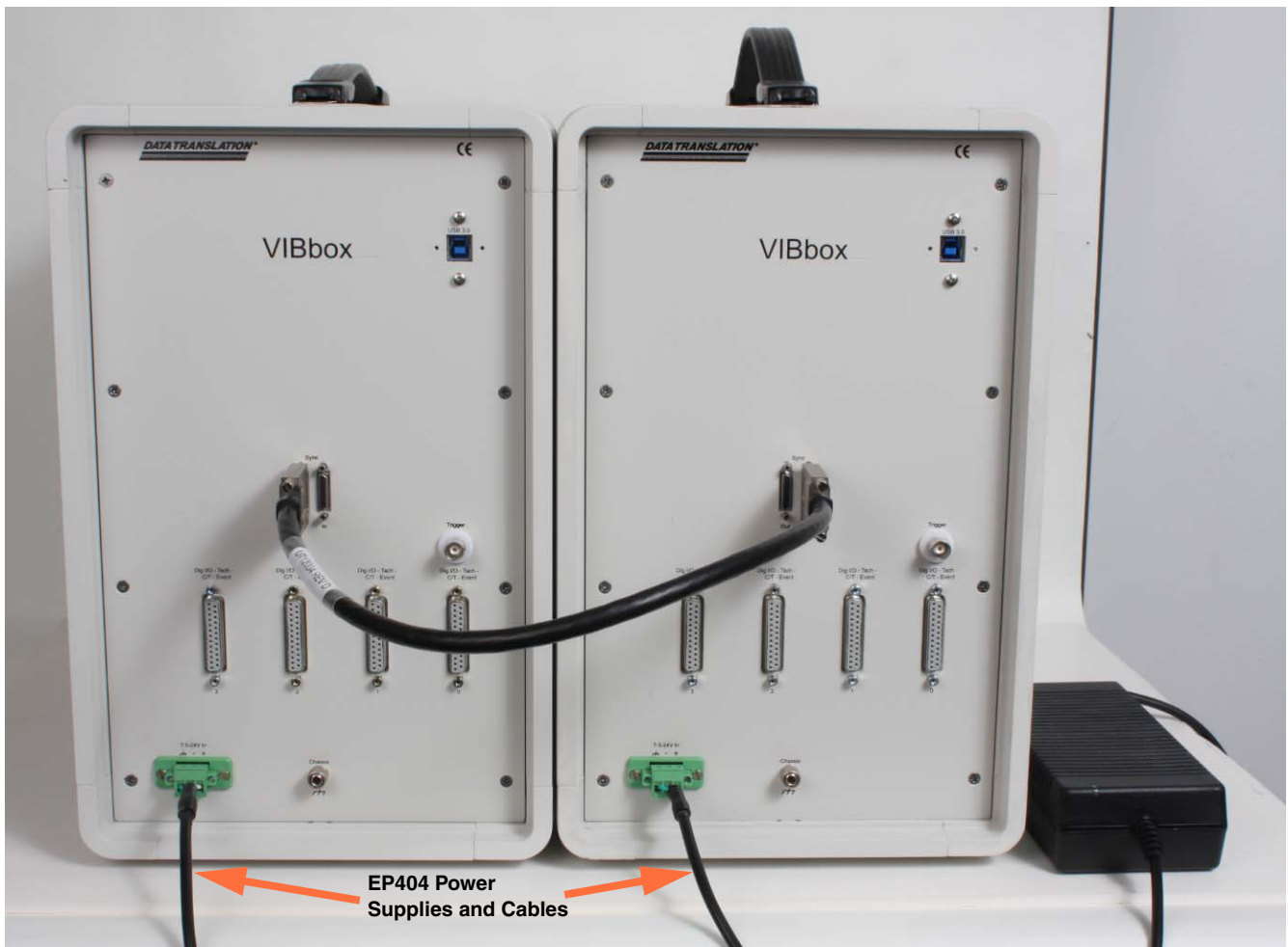
Figure 52: Connect an EP404 Power Supply to Each VIBbox
