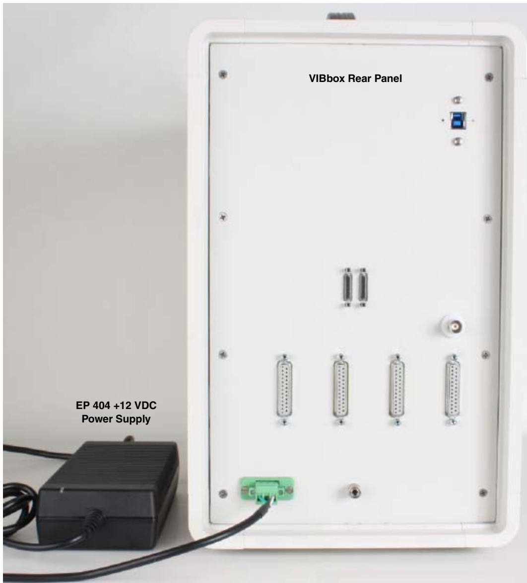
Connect the EP404 Power Supply to the VIBbox and to the Wall Outlet
