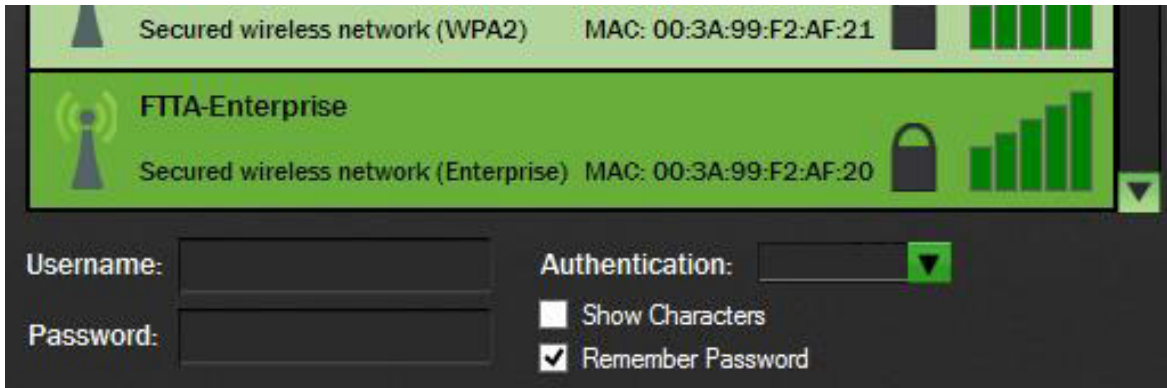
Figure 59: Selecting a wireless network with Enterprise Authentication
