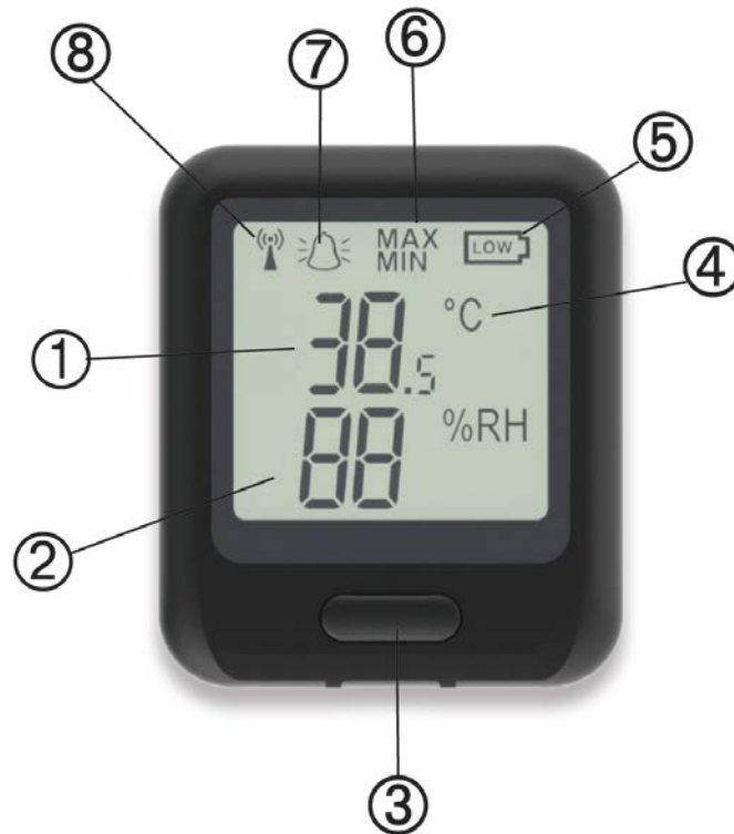
Figure 49: WiFi-500 device components
