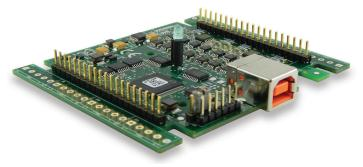
The USB-1608FS-Plus-OEM has the same specifications as the USB-1608FS-Plus, but comes in a board-only form factor with header connectors instead of screw terminals.
