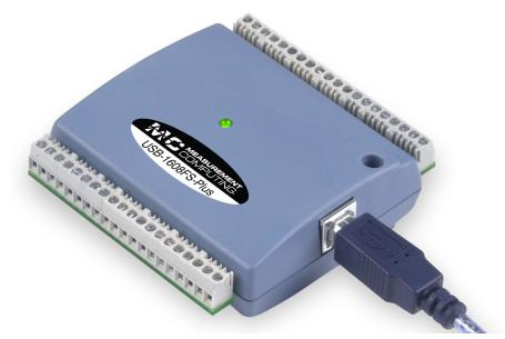
*The USB-1608FS-Plus offers 8 simultaneous analog inputs at up to 100 kS/s per channel (400 kS/s overall), 8 digital I/O, and one event counter input.*
