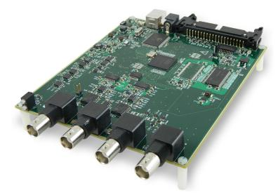
The USB-2020 offers high-speed simultaneous sampling at rates up to 20 MS/s per channel to onboard memory.
