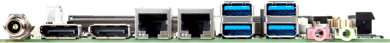
DC Jack DisplayPort DisplayPort GbE RJ45 Ports USB3.0 Ports Mic-In Jack Line-Out Jack
