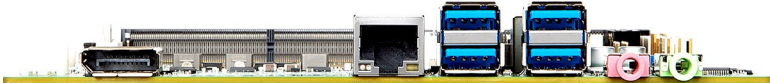
DC-In Connector DisplayPort GbE RJ45 Port USB3.0 Ports Mic-In Jack Line-Out Jack
