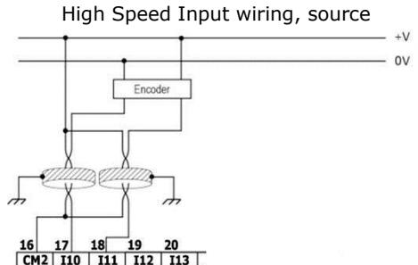
**NOTE** Use sink input wiring to connect a sourcing (pnp) device.
