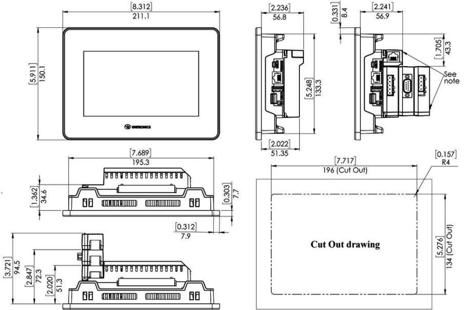
**NOTE** Allow space for modules to be snapped onto the back of the controller, if required by your application. Modules are available by separate order.
