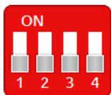
Use the factory default settings (DIP switch 3 and 4 in OFF position).
