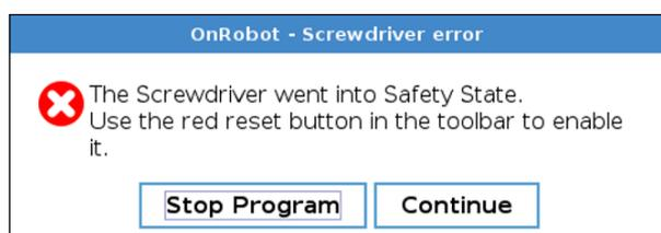
After pressing any of these 2 buttons, the Screwdriver can be enabled by opening the toolbar and pressing the
