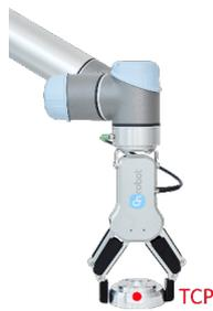
If a tool is attached to the robot, it makes easier for the user to change that point to the tool's "end" point (see illustration on the left).
