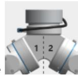
part 1 on the left side and the part 2 on the right side. The numbers are written on the side of the Quick Changer that connects to the robot.
