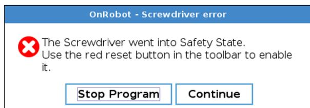
After pressing any of these 2 buttons, the Screwdriver can be enabled by opening the toolbar and pressing the
