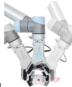
How "far" the TCP needs to be moved to be at the "end" of the OnRobot tools could be found in the [8.3. COG, TCP](#) section.
