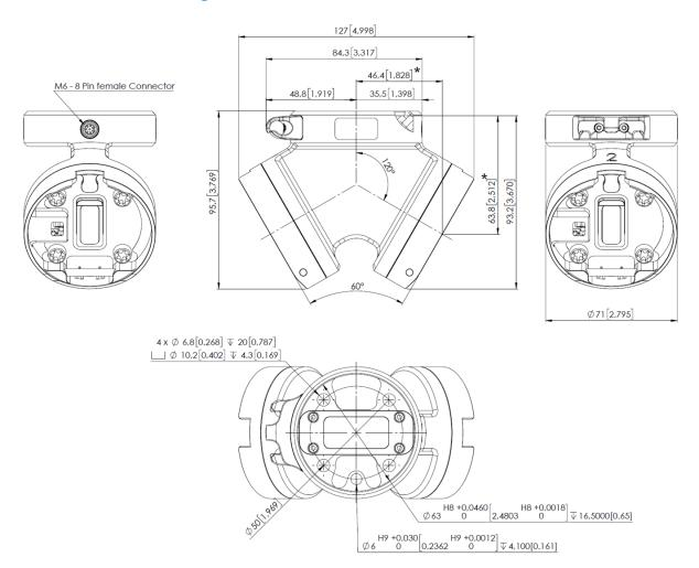
\* Distance from Robot flange interface to OnRobot tool
