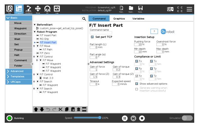
**Gain of force**: The proportional gain parameter of the force control for the side forces on compliant axes.
