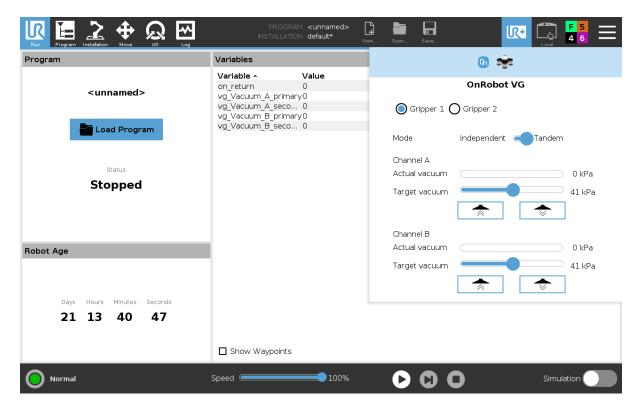
**Gripper 1** and **Gripper 2**: In case of using 2 VG grippers you can select which one performs the action.
