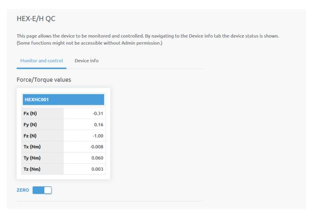
The force and torque values (Fx,Fy,Fz and Tx,Ty,Tz) are shown in N/Nm.
