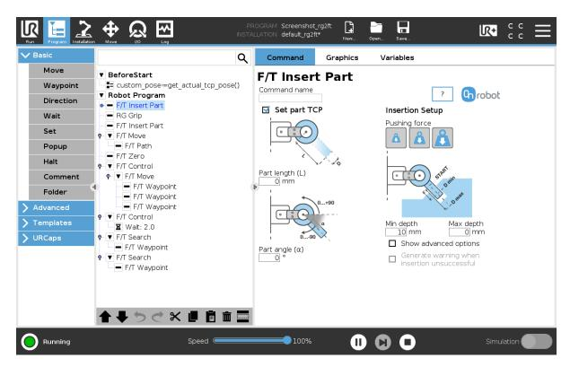
If the **Set part TCP** checkbox is checked the TCP will be set at the further end of the part. It requires the following two parameters to be given:
