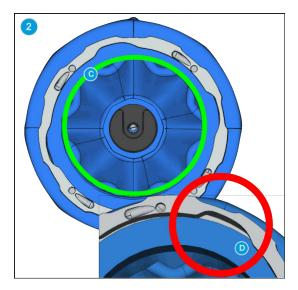
Press the SG tool up against the ring until it fits perfectly **(C)**. Make sure there is no gap between the SG tool and the ring **(D)**.
