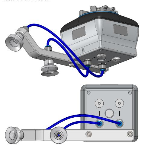
The image below shows how the push-in fittings and the normal fittings are communicated.
