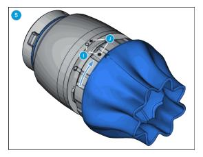
Align the markings (I). Press the SG tool into the SG Base Part and rotate CW to align the two markings (J).
