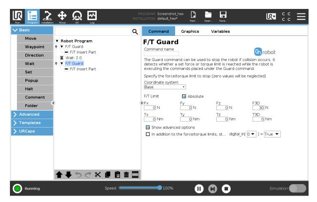
If the In addition to the force/torque limits, stop if is enabled, then the set digital I/O will also be monitored and once the condition is met (along with the force/torque limit) the robot will be stopped. (e.g.: stop if Fz>5 AND digital in\[7\] == True).
