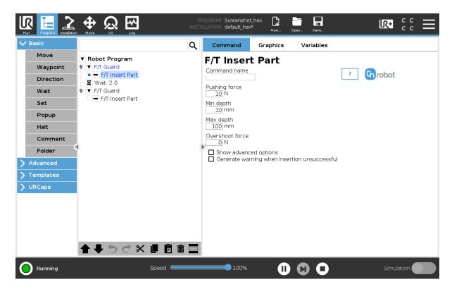
**Pushing force**: The force target used for the force control to gently push the part into the hole.
