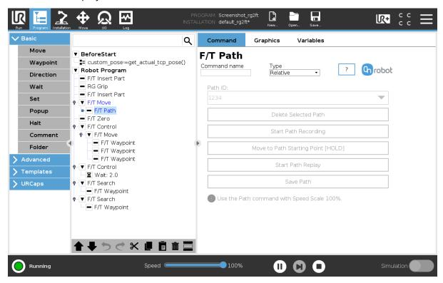
**Type**: If relative is selected, the Path is replayed starting from the actual position of the Tool, instead of the absolute position where it was recorded. If absolute is selected, the Tool moves to the original starting point, and replays the Path from there.
