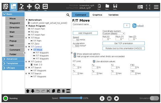
**F/T Limit Fx,Fy,Fz,Tx,Ty,Tz,F3D,T3D**: If any of the values reach the set threshold the stop is triggered. Values equal to zero are neglected. More than one option can be set.
