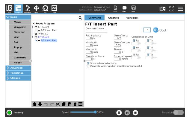
**Gain of force**: The proportional gain parameter of the force control for the pushing force, and the side forces on compliant axes.
