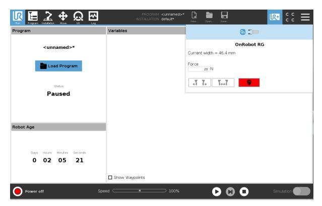
**Gripper 1** and **Gripper 2**: In case of using two RG grippers you can select which one performs the action.
