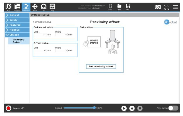
**Calibrated value**: shows the value to use for the application. This value is calculated as the **Raw value** minus the **Offset value**.
