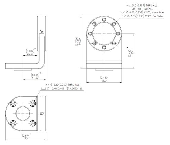
\* Distance from Robot flange interface to OnRobot Quick Changer.
