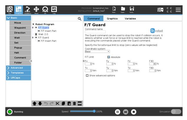
**Coordinate system**: The coordinate system used both for the movement and for the sensor reading. It can be set to Base or Tool (according to the UR's reference frames).
