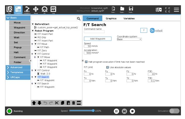
To operate the F/T Search command tap on the **Add Waypoint** button to add an F/T Waypoint as a child node. More waypoints can be added in the same way. To remove a waypoint, use the **Structure** tab **Delete** button.
