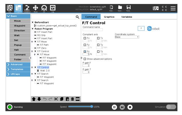
**Compliant axis Fx, Fy, Fz, Tx, Ty, Tz**: The axis selection that needs to be compliant. If an axis is enabled (compliant) the movement along/about that axis is force/torque controlled otherwise (non-compliant) position controlled. The enabled axis is controlled to keep the set force/torque value constant. At least one compliant axis must be selected.
