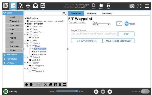
**Target TCP pose**: The position represented by the waypoint in the robot route. It is a readonly field and can be filled by using the **Get current TCP pose** button.
