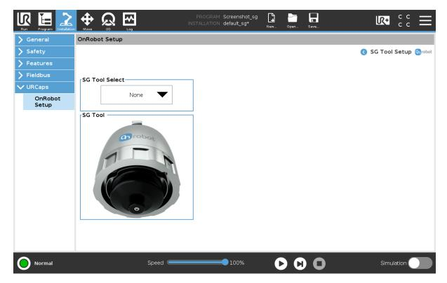
When choosing a tool, in the dropdown menu, the gripper will automatically initialize to the chosen tools neutral position. This will also automatically set the right tool operating parameters such as width, TCP and tool Center of Mass.
