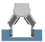
These are open and close hold-to-run buttons. Notice that to enhance width precision the target Force is not applied when using these buttons.
