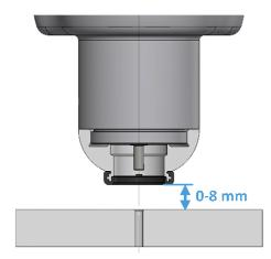
From a safety perspective, this ensures that nothing larger than 8 mm is exposed to be harmed by the Screw-bit System while executing a Screwdriver operation.
