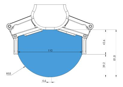
Gripping on long objects can unintentionally activate the Safety switches. The maximum workpiece height (calculated from the end of the fingertips) is dependent on the gripping width (w). For various width values the height (h) limit is given below:
