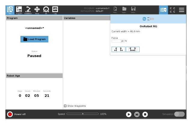
Current width: shows how wide the gripper is opened.
