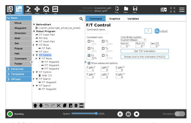
**I gain F**: The force controller can be tuned with this integral gain parameter. If any overshoots or vibrations occur, try lowering the gain value.
