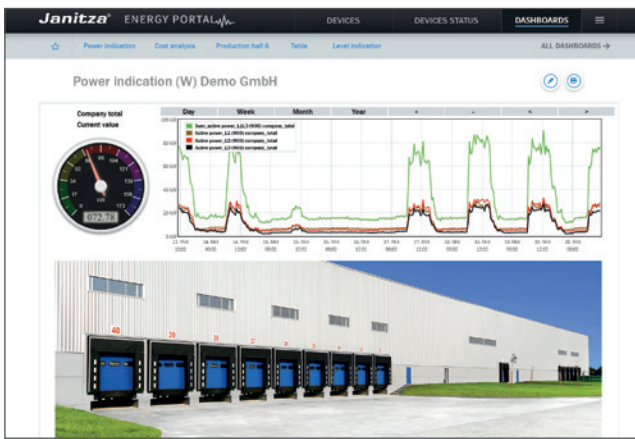
Example of a dashboard with a line chart (load profile) and the power value displayed using an analogue pointer display.
