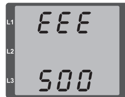
Fig. Warning message with number 500 (mains frequency)
