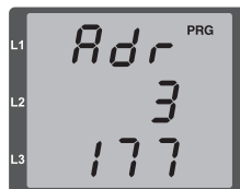
Fig. TCP/IP address Byte 3, value 177
