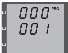
Fig. Parameter screen programming mode Buttons 1 and 2 can be used to modify the individual parameters (cf. page 46).
