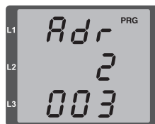
Fig. TCP/IP address Byte 2, value 003
