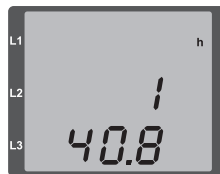
Fig. Measured value screen Operating hours counter
