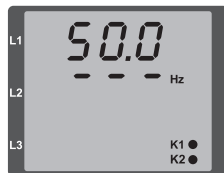
Fig. Direction of the rotating field not detectable.
